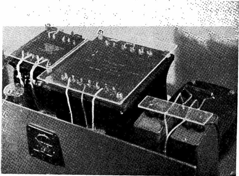
Showing how clear plastic covers should be fitted over all high-voltage components in a power pack. In this case, transformers and smoothing-condenser terminals are covered, making the power pack safe against accidental contact.
