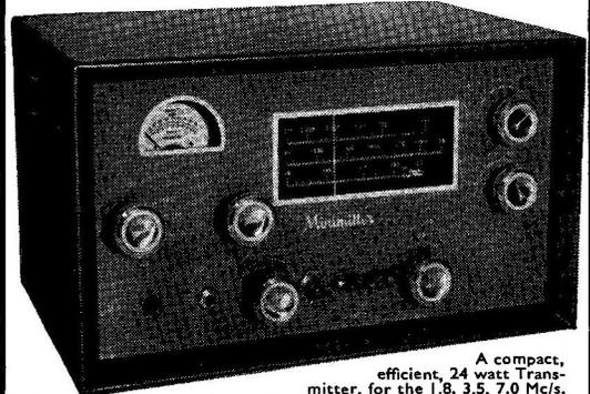
A compact, efficient, 24 watt Transmitter, for the 1.8, 3.5, 7.0 Mc/s. bands. Completely self-contained, with built-in Aerial change-over and control relays — Input and Output monitoring — High Level Modulation — V.F.O. or Crystal Control — Large Slide Rule Dial — complete remote control facilities. Price £30.0.0 Complete
