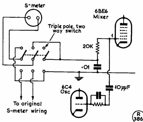
Showing a method of measuring grid current in the mixer stage of a communications receiver fitted with an S-meter, in the circuit as used in an HRO. The grid resistor and bypass condenser should be as close as possible to the mixer valve.
