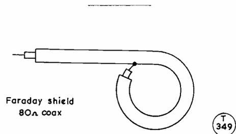
Fig. 3. A screened link winding (Faraday shield) can be made from ordinary coax cable. The end of the inner conductor is soldered to the outer braiding at the start of the link turn — and that is all there is to it.
