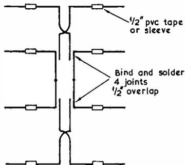
Fig. 3. Radiators and phasing lines
