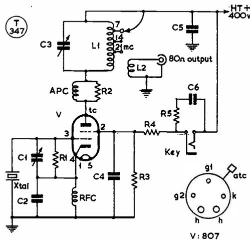
Fig. 1. Circuit of the single-valve transmitter ("one-lung perker" or "junk box special") built by G3BDQ in a couple of hours as a relief from SSB design and constructional problems. This is a simple 20-watt CW job capable of good results on four amateur bands—indeed, it will give world-wide contacts and involves no complications because it is crystal-controlled.
