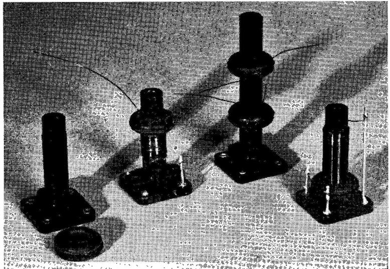
Illustrating the points made by the writer in his article. Push-fit rubber grommets (as used for chassis insulation) secure the windings in place on the coil formers, either temporarily until cementing is completed, or permanently in certain applications. These grommets can also themselves function as coil formers, where coupled windings are required, enabling a close adjustment of mutual coupling to be made.
