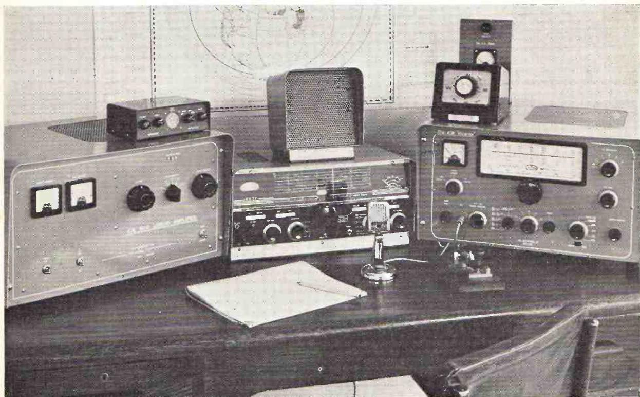
The KW Station comprising (left to right) KW 500 Linear Amplifier, Hammarlund HK1B Electronic Keyer, KW 77 Triple-Conversion Receiver and Speaker, Geloso Table mic, KW Viceroy transmitter, CDR Beam Control Unit, KW Match SWR indicator (Vibroplex bug-key and 'phones in desk drawer).
