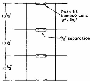
Fig. 6. Bamboo reflector spacers
