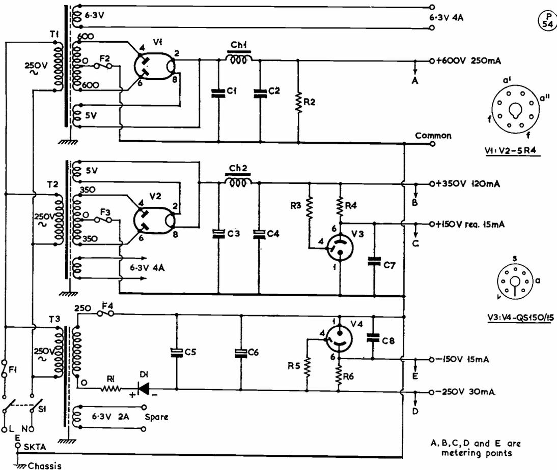
Fig. 1. Circuit complete of the multi-output power supply unit, using three transformers to get all the normally-required voltages for the operation of a transmitter running up to full power on the amateur bands. For a piece of apparatus of this kind, which is in the "fit-and-forget" category, good quality parts should be used throughout, all mounted on a substantial chassis, with proper earthing arrangements.
