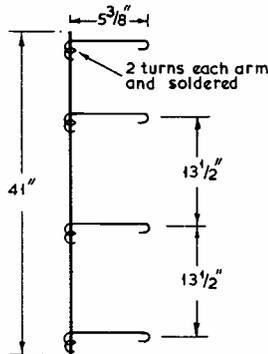
Fig. 4. Element support 2 off
