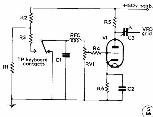
Fig. 1. Circuit for an FSK Keyer, as explained in the text. The 850-cycle deviation is applied to the VFO of the main transmitter. Adjustment is by means of C3 and RV1 for correct operation, and the keyer is driven by the transmitting teleprinter.
