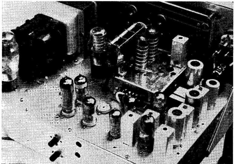
General layout above chassis of the G5NH receiver, using a modified TV-type coil turret as the main tuning unit. Full circuit details are given in the article, and a suggested mechanical layout in Fig. 4. The unfilled valveholder visible in this photograph is for possible circuit extensions.
