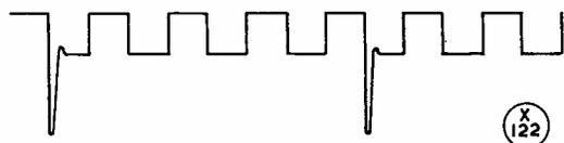
Fig. 2. Referring to Fig. 1, this is the waveform seen on a CRO with the output taken from the monitor point when the blocking oscillator is switched to the 25 kc setting, to give a 4:1 division of the fundamental frequency.
