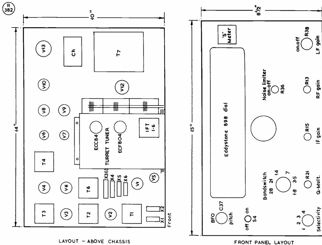
Fig. 4. The chassis and panel layout adopted by G5NH for the receiver described in his article, an impression of the finished appearance being given in the photograph. Since this design is intended to suggest circuit ideas to the more experienced constructor, no great detail is given as to its actual construction and mechanical arrangement.
