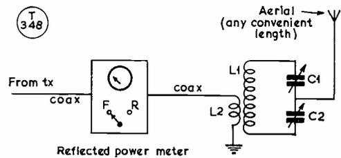
Fig. 2. Suggested ATU arrangement for the simple transmitter, as used by G3BDQ. To obtain maximum efficiency, an SWR or Reflected Power meter should be included on the aerial side, as shown here. The circuit components are: C1, C2, 300  $\mu\text{F}$ ; L1, plug-in coil for the band; and L2 is a single-turn Faraday link, as shown in Fig. 3.
