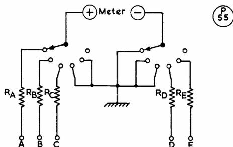
Resistors  $R_A$  to  $R_E$  should be fitted under the chassis on a suitably insulated tagboard
