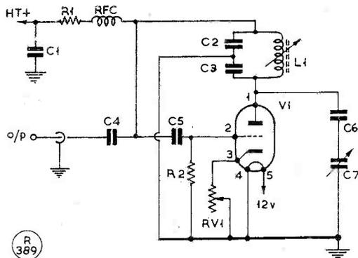
Fig. 2. Q-multiplier arrangement used by GW8PG for his TCS receiver — and see Fig. 1 for inter-connection. C7 is the peaking condenser. The selectivity of the receiver is considerably improved by incorporation of this unit.
