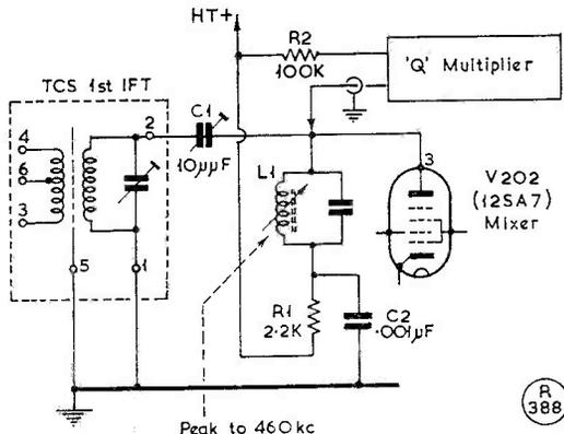
Fig. 1. The IF circuit modifications for the TCS receiver, discussed by GW8PG in the text. C1 is for bandwidth control.
