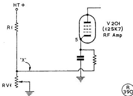
Fig. 3. Separating the RF and IF gain controls on the TCS receiver. In the original, this is common to both, as in many surplus types. The modification is explained in the text, and values here are 220K for R1, and 20K for RV1.
