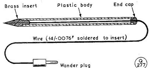
The sketch shows a cross-section of the assembly. A test lead of this nature should fill the needs of those in a similar predicament, and would also serve those who have constructed test meters described in this *Magazine*—all of which articles never mention a test prod!
