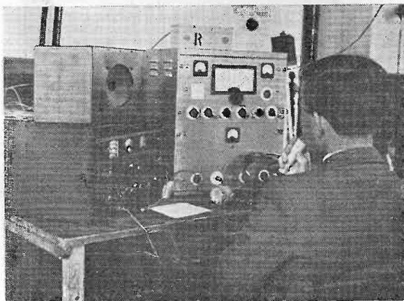
The Top Band talk-in station for the Cornish Radio & TV Club's Rally at Penzance over June 15-16 ran a Tiger-100 Tx (throttled back for 160m., of course) and an AR88 Rx, the aerial being an 8 ft. centre-loaded whip. In this picture, G3RID is operating.
