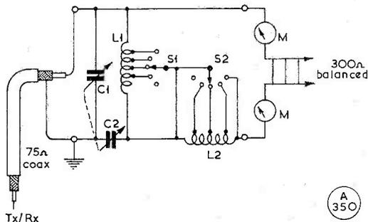
Fig. 2. A multi-band adjustable balun for the HF ranges, which can be used either way round. Values are given in the text, opposite.
