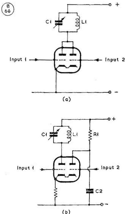
Fig. 3. Double-triode mixers are suitable both for receiver work or for the early stages of transmitters. At (A) the anodes are paralleled and the combined frequency selected by the tank circuit L1, C1; at (B) the second anode is held at earth potential (RF) by C2, so that the second half of the triode runs as a cathode follower, with a common cathode load.
