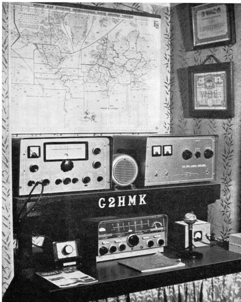
installation, and likewise is for SSB working only. It consists of an AR88D receiver and the transmitter is a home-constructed G5BJ-type crystal filter exciter into a 6AG7 buffer driving a TT21 linear running about 50 watts; this in turn pushes an 813 linear PA to full p.e.p. on 20 and 80 metres. The aerials used, for either station, are an 80-metre dipole and a Mosley TA-33JR. beam.
