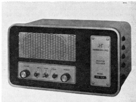
This is an example of the new Hammarlund range of monitor receivers, intended for crystal-controlled fixed-frequency working in the amateur and commercial bands 25-54 mc and 144-174 mc. Selection of up to six channels is provided by panel control, for either NBFM (5 kc deviation) or WBFM (15 kc deviation) depending on model used and service required. The main application of these receivers is in government communications services and on business or industrial radio networks.
