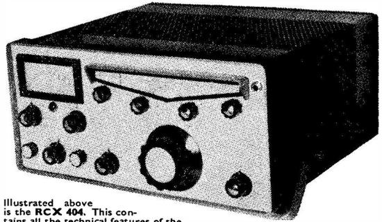
Illustrated above is the **RCX 404**. This contains all the technical features of the **RCX 202** plus the maximum possible crystal stability together with a kilocycle counter that can be read to within 500 cps. with ease, and a tunable Band Pass input filter stage for the maximum rejection of strong unwanted signals. This is a Receiver with wave-meter accuracy for the connoisseur. Price £135 — also available with any 12 500 kcs. sections in the frequency spectrum .5 mc/s. to 30 mc/s. Price £145
