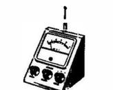
3 bands 2.5 to 57 mc/s., permits easy tune up for max. transmitter output. Earphone jack to monitor audio. 200µA meter cal. 0-10. Supplied complete with battery, telescopic aerial, £7/7/- each. P.P. 2/6.
