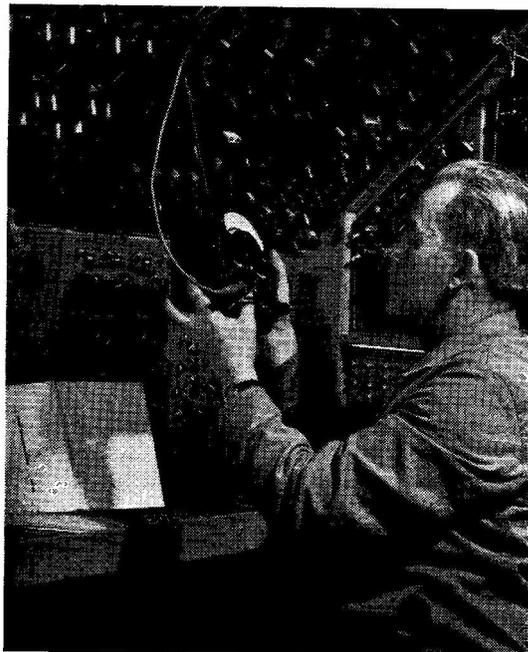
A B.A.C. technician using the Model 8 Mk. III test-meter, the latest instrument in the AVO range, to go through the flight engineer's panel on a VC-10 jet aircraft. Its layout will give any AT-station operator ideas about the economical use of space; there is a vast amount of circuitry behind those panels in the cabin roof.
