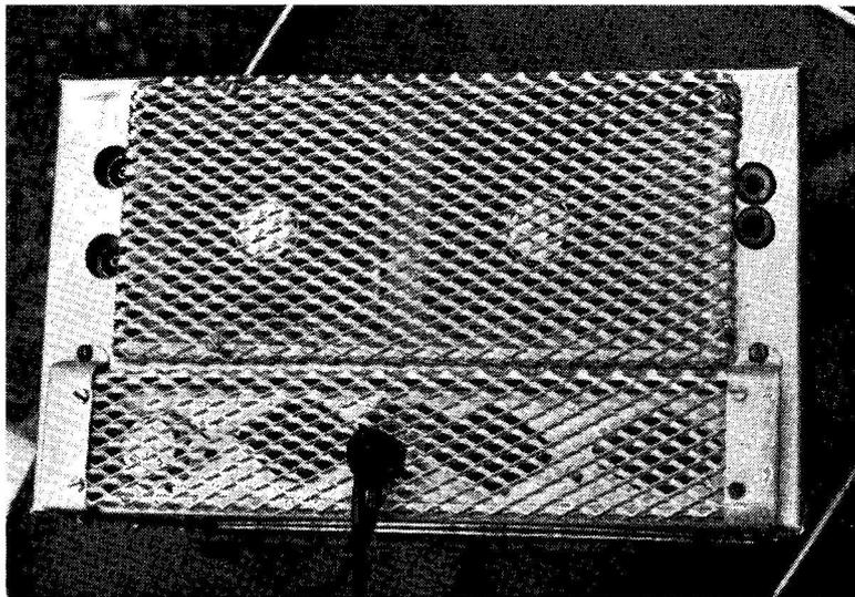
Rear view of the EI7A 80m. TTx, running a good 30 watts, fully modulated, using transistors only. Since those mounted on the rear panel dissipate some heat, speaker grille material is fitted to provide ventilation.
