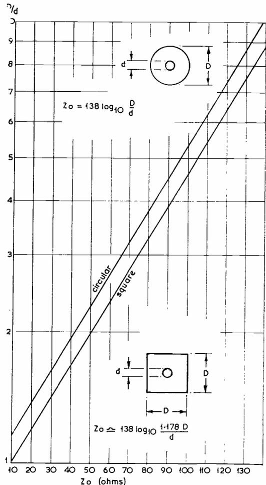
Fig. 1. Ratio of inner conductor diameter to outer conductor dimension, D/d, plotted against impedance, Z<sub>0</sub>, for both square and circular outer conductor.
