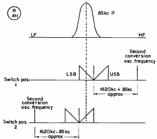
Fig. 1. The 85 kc IF channel can be produced by placing the conversion oscillator either HF or LF of the first IF. By switching from one frequency to the other, the sidebands are transposed, so that either the upper or lower sideband will appear in the IF pass-band.
