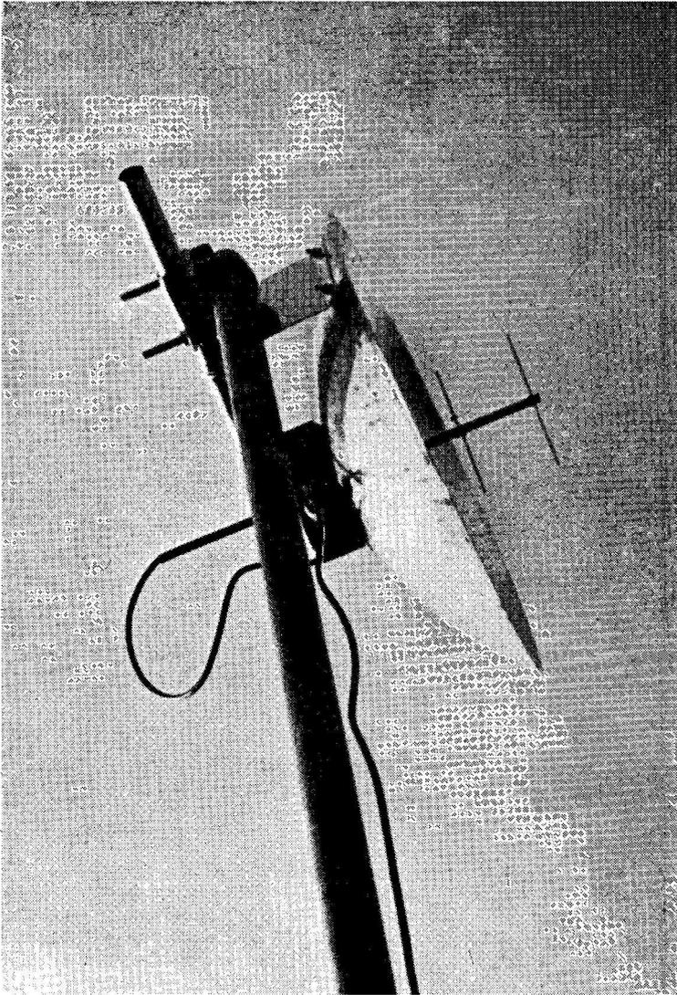
For a VHF/UHF field test over October 18-19, the Bristol Amateur Radio Club (signing G3OUK) had a 2ft. parabolic reflector system consisting of a driven element with a parasitic lug, tuned into the 23-centimetre band. On this, they heard GW3ATM (Chepstow) in contact with G3MPS (Bridgwater) on 1296 mc. Their equipment consisted of a half-wave trough-line on a CV-291 as mixer, with an ECC85 as head amplifier. No actual 23-centimetre contact was obtained.
