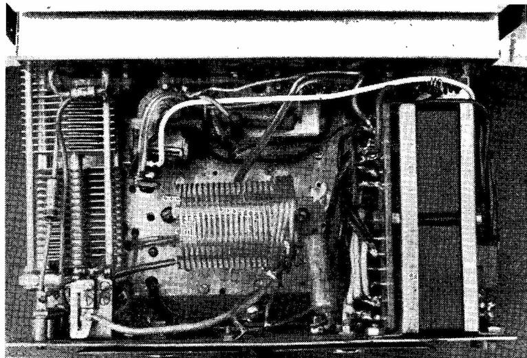
Upper chassis view of the 30w. transistor Tx, showing the PA tank assembly; the coil, L3 in the diagram, has been made high-Q and its constructional detail is given in the Table of Coil Values. In this picture, the modulation transformer T3 is to the right, and the mounting for the four meters (out of their cases) is visible along the top of the photograph. The 2N1046's in the PA are mounted with cooling fins.
