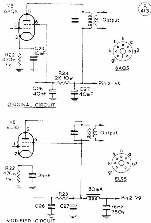
Fig. 1. The original output end of the HE-30, as modified by G3GDJ and explained in the text.
