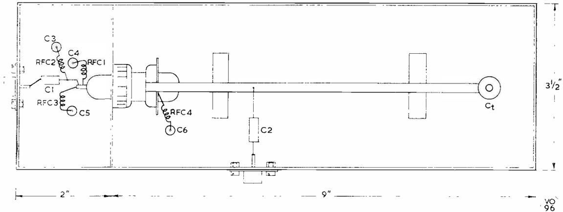
Fig. 2. This sketch is to almost exactly half-size, and shows the mechanical layout of the circuit of Fig. 1. The valve is a disc-seal triode, type DET-22, in which the grid connection is made to a copper ring, this forming the earthing point when the valve is mounted in the screening panel. The depth of the trough is two inches, and other details are given in the text.
