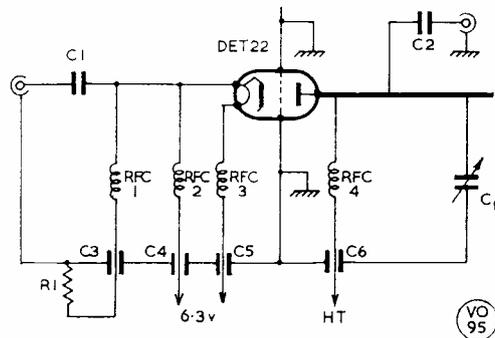
Fig. 1. Circuit of the 70-centimetre pre-amp. described by G3NDC, using a DET-22 in grounded grid. A physical layout for the trough, with dimensions, will be found in Fig. 2.
