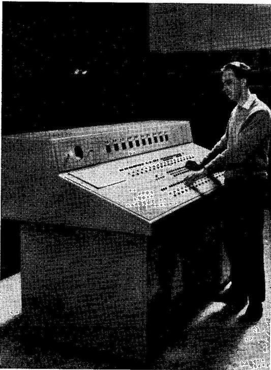
The control console for the 36 aerials in the Radio Australia radiating system, giving world-wide coverage and directivity as required. Aerial system, transmitter and frequency can be switched in a matter of seconds.
