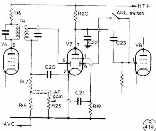
Fig. 2A. The original circuitry involving the detector and AVC line in the HE-30. Some suggested modifications are shown in Fig. 2B. It should be noted that the circuit designations are in accordance with the manufacturer's handbook on the receiver.
