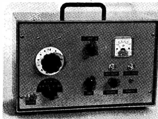
The new "Telecomm." Portable Field Strength Indicator and Test Set, type FS8/T. It covers all channels in the TV Bands I and III, with display on a robust m/c meter. The instrument is designed round a transistorised superhet circuit, powered by two 6V, PP1 batteries, on which the total load is only 30 mA, to give months of life. The channel selector switch brings in Ch. 1-13, and other controls are for fine tuning, output control and pre-set zero adjustment.
