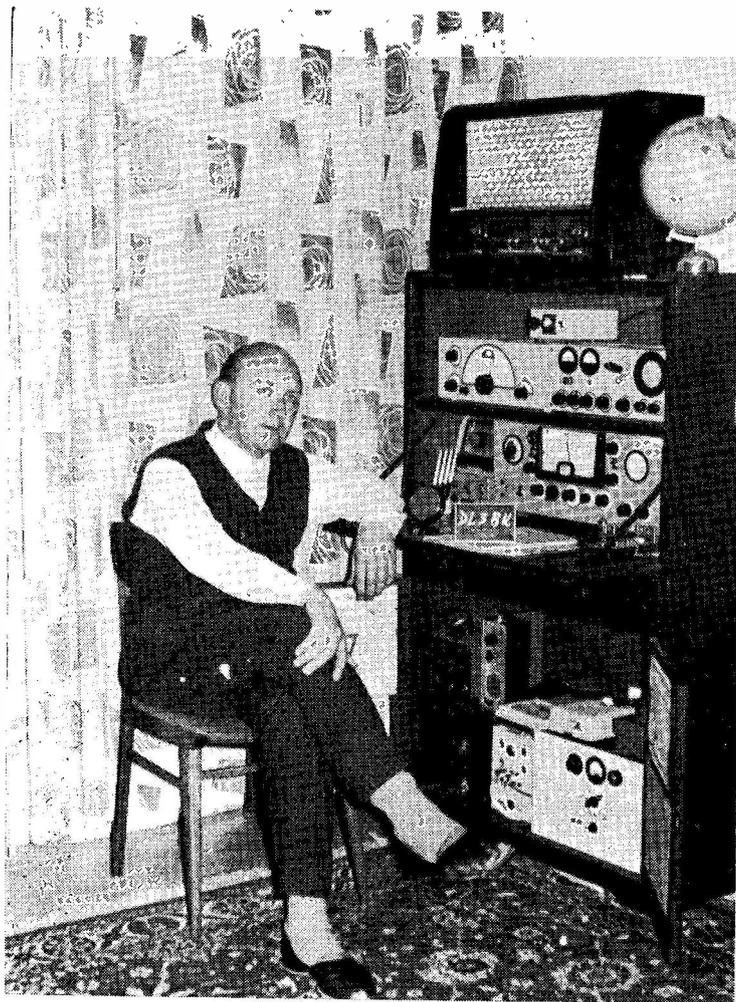
Station of DL3BK, Hans Scholz, Ackermannstrasse 31, Stuttgart, consisting of a 200w. Tx, a double-conversion superhet receiver and, outside, a 3-band Quad — and all this lot is entirely home-constructed.
