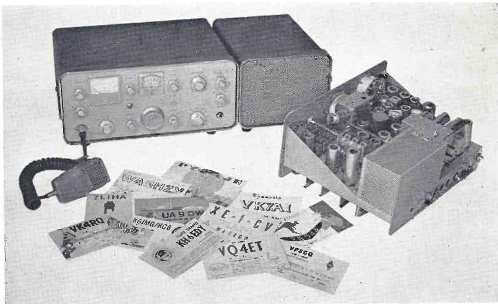
The KW 2000 SSB Transceiver is now available on short delivery. SSB and CW, 10-160 metres mobile or fixed station. Voice control, built-in crystal calibrator, etc. A complete station costing £199.
