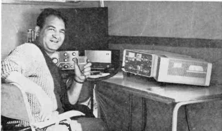
For the Red Cross Gala at Chelmsford on June 26, the Amateur Radio Mobile Society kitted out a very effective station, using a KW-2000A loaned by K.W. Electronics, Ltd.; a Swan-350, provided by K6IWG; and a Hy-Gain 16AVO vertical aerial. World-wide contacts were made and the station, here seen operated by G3NMR of A.R.M.S., was a continual focus of interest for the public. Talk-in was also provided, using separate stations, on two metres and 160m. *Picture by G3NMR.*
