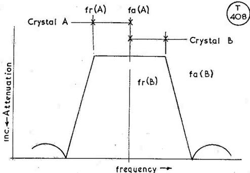
Fig. 5. The theoretical attenuation curve of a filter using two crystals, where the "fa" of the lower frequency crystal is the same as "fr" in the higher frequency crystal.
