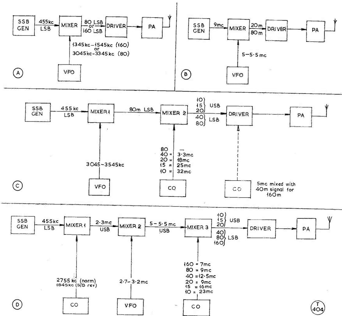
Fig. 1. Some typical configurations for SSB transmitter layouts. (A) Single-band transmitter for 80 or 160 metres. (B) A two-band Tx for 20/80m. (C) Five or six band transmitter with automatic Sideband selection. (D) A six-band Tx with automatic Sideband selection plus the facility for switching sidebands without changing frequency.
