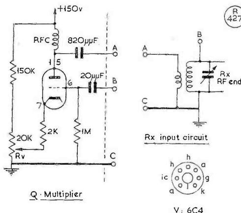
The circuit shown here, applicable to any receiver in which the "B" point is accessible, can have the effect of narrowing the Rx bandwidth at the input end. Thus, it will improve image rejection—particularly in the case of receivers having no RF stage before the mixer—and also signal-to-noise ratio.
