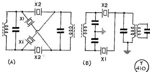
Fig. 7. Showing at (A), a full-lattice crystal filter, and at (B) a half-lattice filter.
