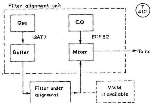
Fig. 9. Block diagram of a suitable set-up for LF filter alignment. The derivation of this arrangement is shown in detail in Fig. 11.
