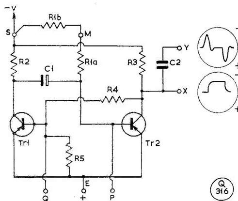
Fig. 1. Monostable circuit for producing dot-and-dash pulses. Timing, in the sense of "dot-dash-space," is determined by the values of C1, R1A and R1B. The wave-shapes shown here should be sharper in outline.
