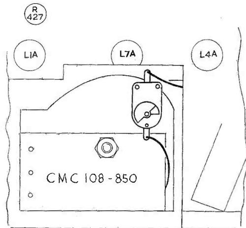
Fig. 2. Rear of the 52 Rx chassis, with the position of the third trimmer for bandspreading indicated — see text.
