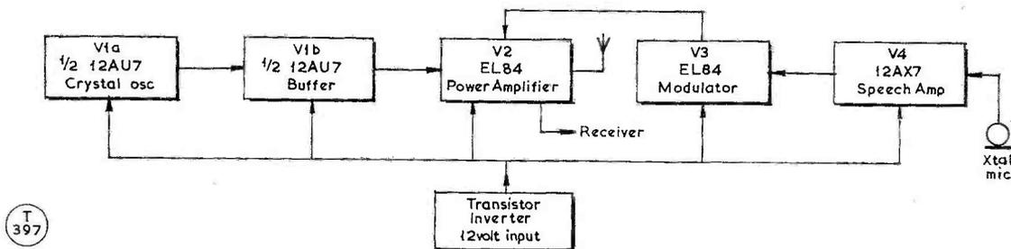
Fig. 1. Block diagram of the complete 160-metre transmitter and modulator, as described by G3JBU. It is a perfectly straightforward arrangement (and therefore sure-fire), and the crystal oscillator driver can be switched to give a choice of several spot frequencies in the Top Band area.
