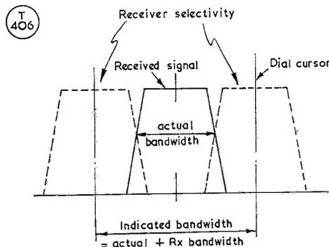
Fig. 3. When attempting to give, over the air, reports on the bandwidth of a Sideband signal, subtract from the indicated figure the bandwidth of the receiver filter.
