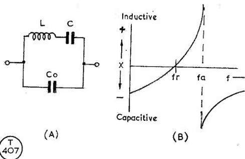
Fig. 4. At (A) is shown the equivalent circuit of a crystal. (B) is a reactance-against-frequency plot of a quartz crystal.
