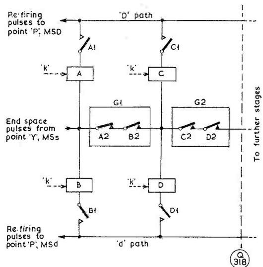
Fig. 3. Showing how paths for either a dot or a dash are preselected by the "K" pulse, as explained in the text. This particular diagram is "for explanation only," and is a logic model to illustrate the working of the system.
