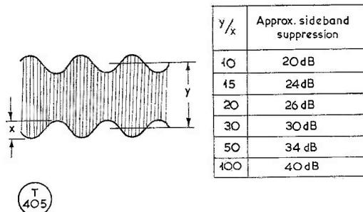
Fig. 2. Method of approximating Sideband suppression of a tone-modulated transmitter by displaying its output on an oscilloscope.
