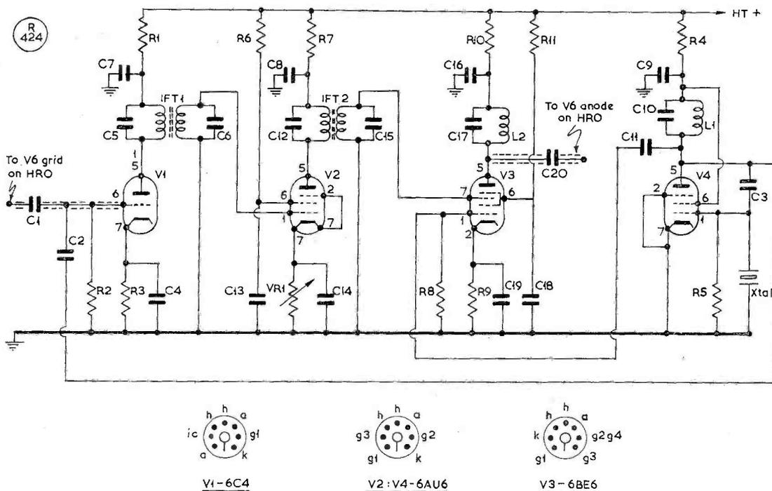
Fig. 3. A suitable Q5'er to work with any HRO in the ordinarily available surplus category. Giving vastly improved selectivity, it can be built separately as an "outboard" unit, and run from the PSU shown in Fig. 1, p.654, January. Details are discussed in the text, and all values are in the table with this diagram.
