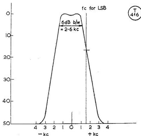
Fig. 13. The passband to be expected from two half-lattice sections cascaded as in the circuit of Fig. 12. The Sideband attenuation could be: at 300 c/s, 24 dB; at 500 c/s, 31 dB; and at 1 kc, 50 dB.
