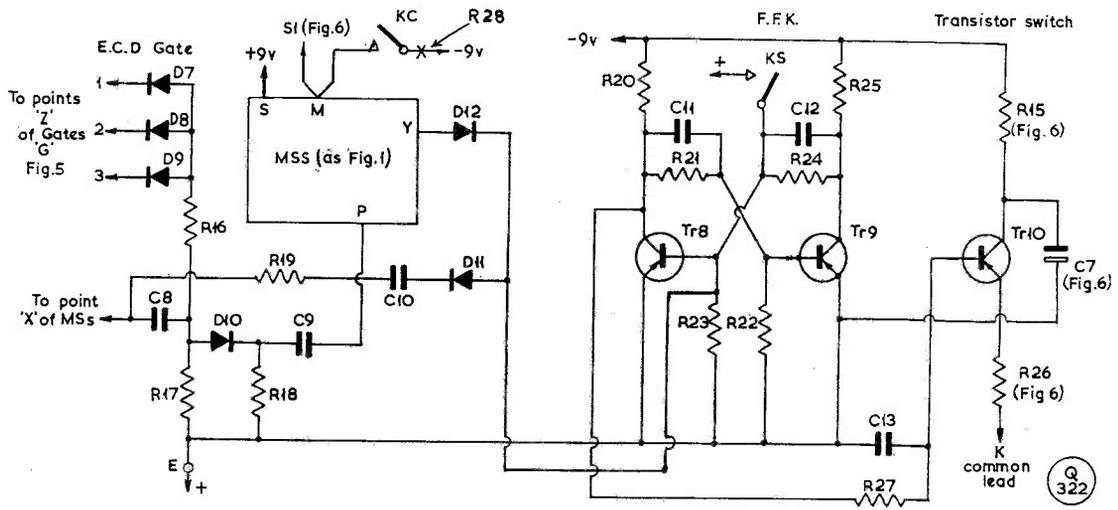
Fig. 7. Circuit for obtaining the inter-character space, as explained in the text. Values are given in the table on p.747 and are applicable to all circuits shown.
