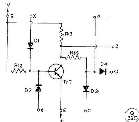
Fig. 5. Transistor gate circuit, performing the function of the contacts A2-B2 or C2-D2 in Fig. 3. This part of the circuit as a whole can be called "an inter-element gate." Point X connects to the X-point in Fig. 4.
