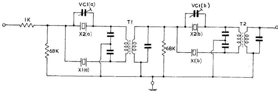
Fig. 12. The question of the filter arrangement to use can be complicated. There are various possible arrangements, as discussed by G3RNL in his text. The layout here is for two half-lattice filter sections in cascade.
