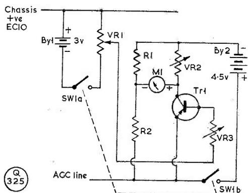
Circuit for an S-meter suitable for a transistor receiver, to give forward reading by reversing the AGC drive voltage. Values are: R1, 100 ohms,  $\frac{1}{2}$ w.; R2, 2200 ohms,  $\frac{1}{2}$ w.; VR1, 10K variable; VR2, 10K variable, zero set; VR3, sensitivity control, one megohm (see text); B1, 3-volt battery; B2, 4.5 volt; M1, 0-1 mA meter; and Tr1, OC81M transistor, or similar.
