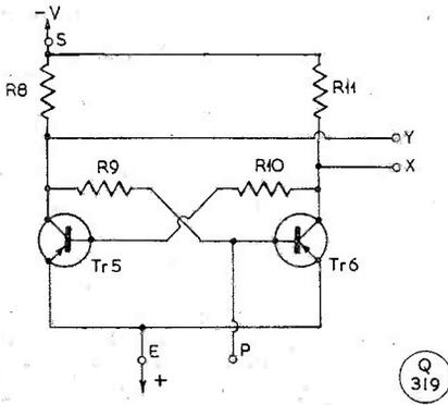
Fig. 4. A bistable, or flip-flop, circuit, actuated by either positive or negative pulses, and working in the same way as the relays in Fig. 3 — only much faster and more positively.
