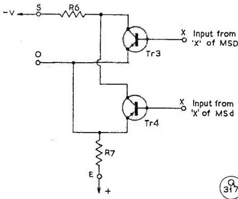
Fig. 2. A transistor switch, producing either a dot or a dash — see text.
