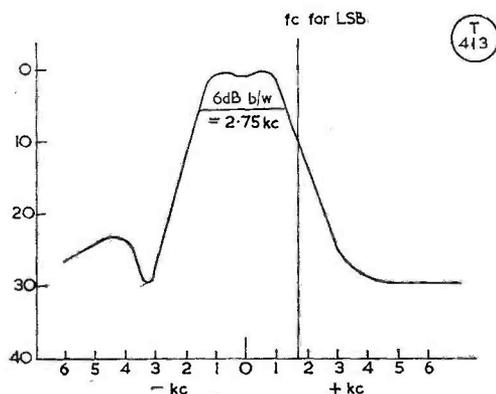
Fig. 10. Plotted passband of the half-lattice filter shown in Fig. 8, when aligned for LSB. The attenuation at 300 c/s is 19.5 dB; at 500 c/s, 22.5 dB; at 1 kc, 27.5 dB; and at 1.5 kc, 28.5 dB. See text.
