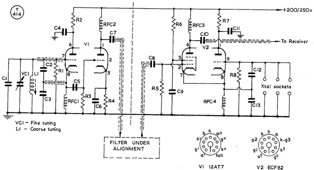
Fig. 11. Circuit of the set-up used for aligning the LF filters. Values are: C1, 150  $\mu\text{F}$ , silver mica; C2, .001  $\mu\text{F}$ , s/m; C3, .002  $\mu\text{F}$  s/m; C4, C6, C9, C11, .01  $\mu\text{F}$ ; C5, C7, C8, C10, 150  $\mu\text{F}$ ; C12, 25  $\mu\text{F}$ ; C13, 250  $\mu\text{F}$ . R1, R3, R5, R8 47,000 ohms; R2, R7 10,000 ohms; R4 2,200 ohms; R6 100,000 ohms. RFC's 1-4, 2.5 mH RF chokes. Tuning VC1, 100  $\mu\text{F}$ . Valves V1, 12AT7; V2, ECF82.
