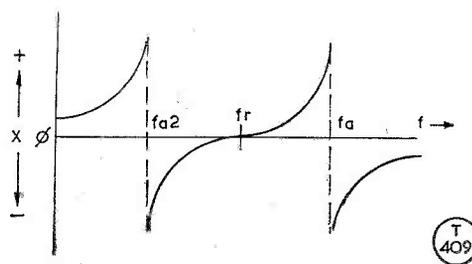
Fig. 6. The reactance/frequency plot of a quartz crystal shunted by an inductance — see text.
