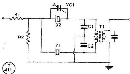
Fig. 8. Practical circuit for a half-lattice filter suitable for use in the fixed-frequency Sideband generator shown on p.664 of the January issue of "Short Wave Magazine." For proper operation, crystal frequency X2 should be about 2 kc higher than X1. Suitable pairs can be extracted from the data given in Table I on p.742.
