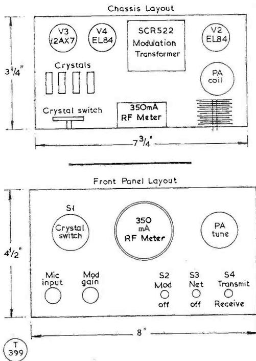
Fig. 3. Suggested panel and chassis layouts for the 160-metre transmitter described by G3JBU. Other arrangements are, of course, possible but with a valve-type Tx, this is as economical of space as any.
