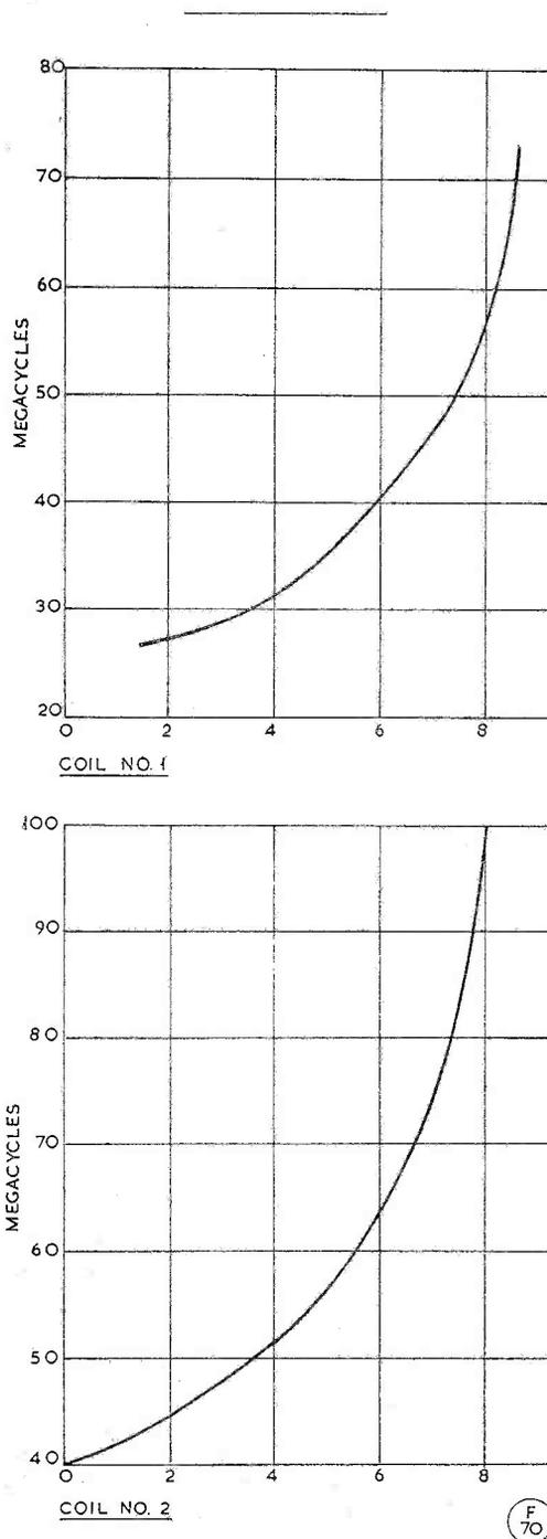
Fig. 2. The calibration curves obtained with the two instruments in the photograph and described in the article. They give a total frequency coverage of 20-100 mc, suitable for much checking work on the HF and VHF ranges. Coverage could easily be extended to 160 mc or so, to take in the two-metre band.
