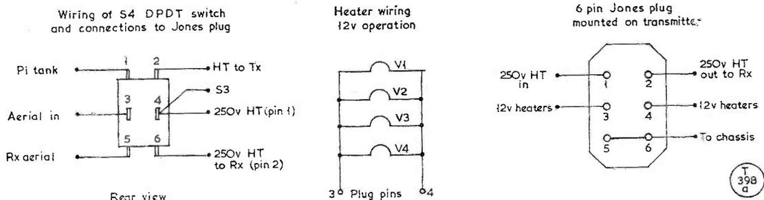
The HT/LT and plug connector wiring for the Mobile transmitter.
