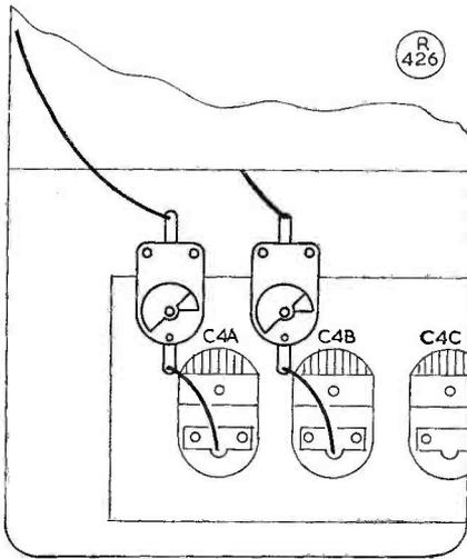
Fig. 1. Side of the 52 Receiver chassis, showing two of the additional trimmers required for bandspreading.
