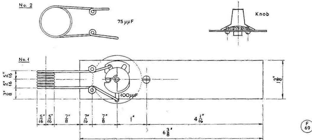
Fig. 1. Mechanical arrangement for the instrument discussed in the text. The No. 1 coil consists of 6 1/2 turns of 16g. wound on a 1/4 in. mandrel (for shape only) spaced out to a little over 1/4 in. The No. 2 coil is of 1 1/2 turns, shaped on a 1 in. former, and spaced out to about 1/4 in. The mounting handles are of perspex, with the edges taken off for easy holding. These wavemeters can be quite accurately calibrated and readings are taken by indirect indication—see text.
