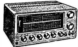
Build this wonderful receiver and save pounds. Supplied semi-completed, main components ready mounted, RF section already wired and aligned. Full and precise instructions supplied. Specifications — 8 valves plus rectifier, 4 bands covering 550 Kc/s.—30 Mc/s. Incorporates 1 R.F. and 2 I.F. stages, 'Q' multiplier, B.F.O., A.N.L., 'S' meter, bandspread, aerial trimmer, etc. Operation 115/230v. A.C. Price 25 gns, carr. 10/-.
