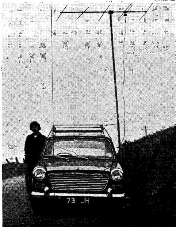
The GM5UM/P set-up for two-metre operation during his recent safari. The aerial mast is a tight fit through a hole in a flat dural plate clamped to the roof-rack by wing nuts, and the butt end of the mast goes through the central hole of one of those large wooden reels on which wire is wound; this makes a firm base, and the beam is easily turned. During the trip, May 29 to June 9, 23 contacts were made on 145.8 mc, from Argyll and Wigtown shires, running 9w. on CW and 7 watts on telephony.
