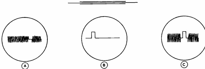
Figure 2. Use of Oscilloscope for Phasing.
