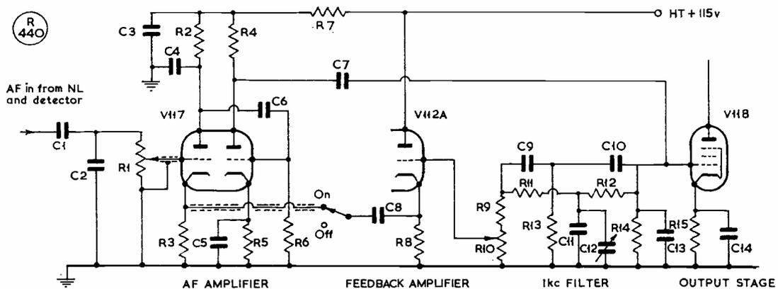
Fig. 2. Circuit of the R.C.A. AR-8516L Feedback Amplifier.
