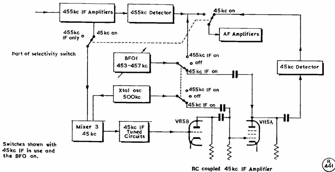
Fig. 3. Beat Frequency Heterodyne System for Dual IF Operation, Bands 3-18 only—see text.
