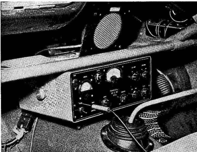
The 80/160m. Transceiver for mobile, designed and built by G3JFH (Cheltenham), well known at Mobile Rallies up and down the country. The transmitter can run up to 40w. p.e.p., from a transistorised PSU. This picture shows how neatly the rig has been constructed and fitted.
