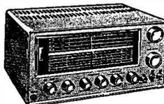
Build this wonderful receiver and save pounds. Supplied semi-completed, main components ready mounted, RF section already wired and aligned. Full and precise instructions supplied. Specifications:— 8 valves plus rectifier, 4 bands covering 550 Kc/s.—30 Mc/s. Incorporates 1 R.F. and 2 I.F. stages, "Q" multiplier, B.F.O., A.N.L., "S" meter, bandspread, aerial trimmer, etc. Operation 115/230v. A.C. Price 25 gns, carr. 10/-.
