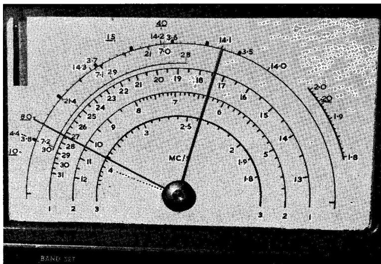
unmarked semicircle replaced the 10-0-100 bandspread reference. Some 1/16in. paxolin was cut to back the scale, and a slot for the EM84 was made in both. The dial was then replaced, without covering glass.
