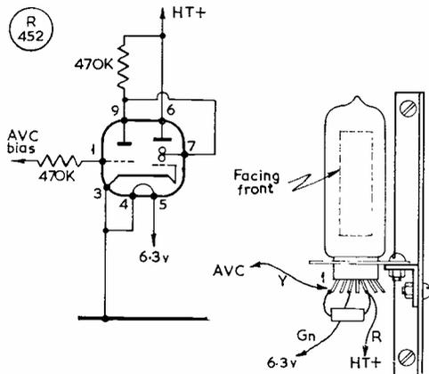
Fig. 1: Circuit and layout for EM84 tuning indicator
