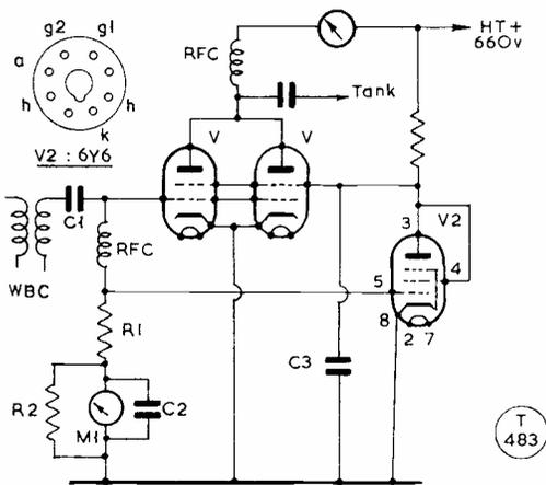
Fig. 1. A typical RF power amplifier circuit using a pair of 807's in parallel, with V2 as the clamper. The usual pi-network tank is assumed.
