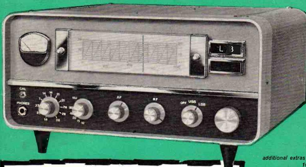
The KW 201 has been specifically designed for optimum performance on Single Sideband. 11 ranges give coverage in the amateur bands from 1.8 mc/s. to 30 mc/s. A mechanical filter gives an i.f. selectivity of 3.1 kc/s. at 6 d.b., and 6 kc/s. at 60 d.b. A 'Q' multiplier is available giving a variable range of 3.1 kc/s. to 200 cycles selectivity.
