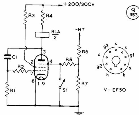
As explained in the text, with the values given here a 40-second pause can be obtained before the relay answers. Since the delay is controlled by C1, R1, it is variable over wide limits—see text.
