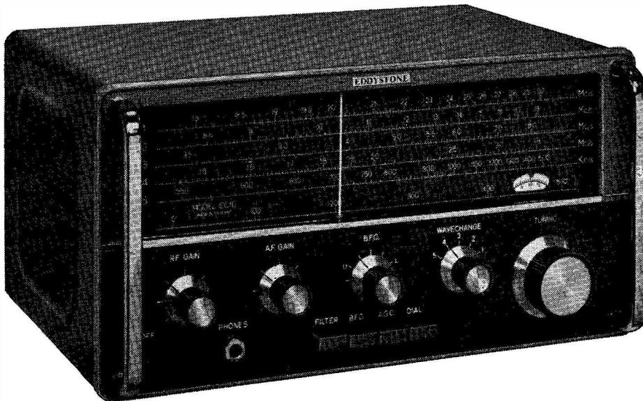
Covering the 1.5 to 3.0 MHz maritime band and providing the maximum listening pleasure from medium-wave programmes, the fully tropicalized EC10 gives reliable reception, in any part of the world, of shortwave broadcasting, amateur, aeronautical and other services in the range of 550 kHz to 30 MHz. The 9-inch tuning scale has a calibration accuracy better than 1% while the logging scale and auxiliary vernier enables station settings to be recorded.
