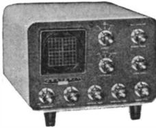
**SB-610E Signal Monitor Scope** . . . operates with transmitters on 160 through 6 metres at power levels from 15 watts through 1 kw. Shows transmitted envelope. Operates with receiver IF's up to 6 Mc/s. showing received signal waveforms. Spots over-modulation, etc.
