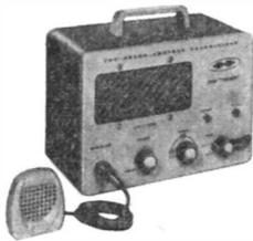
**HW-30 2 Metre Transceiver** . . . For fixed, portable, or mobile. Ideal for local and RAEN purposes. Input 5 watt. CC. Tunable regenerative RX. Size 9 3/4" w. x 8" h. x 6" deep. (For 230v. operation if required).
