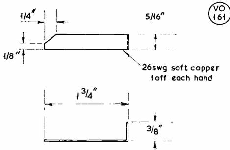
Fig.4: QQVO2-6 LINES (L5) 13cm CONVERTER
