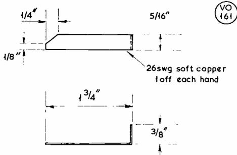
Fig.4: QQVO2-6 LINES (L5) 13cm CONVERTER
