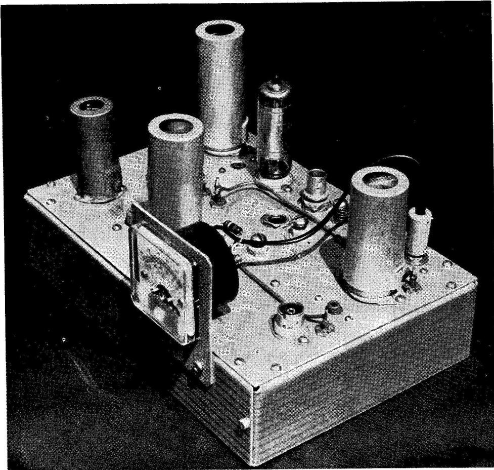
**T**HE converter to be described was developed some four years ago for use on the 13 cm. band. The design was inspired originally by the 23 cm. K6AXN converter which had been in use at the home station for some years and had proved very reliable. The aim was to build a 13 cm. converter using a minimum of stages and comparatively small in size which could be used for portable and fixed station use. A further necessity was to include arrangements whereby the converter could be easily
