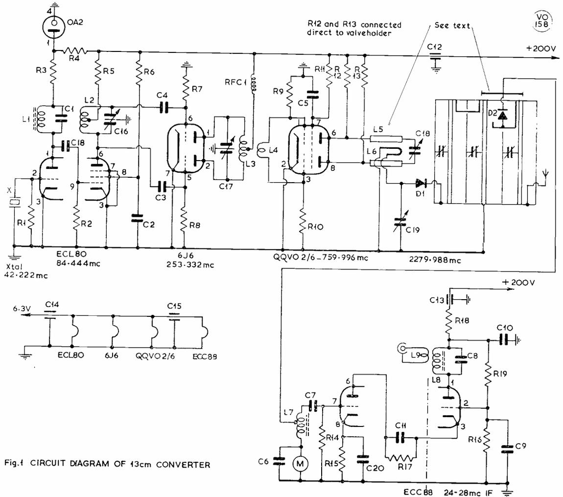
Fig.1 CIRCUIT DIAGRAM OF 13cm CONVERTER
