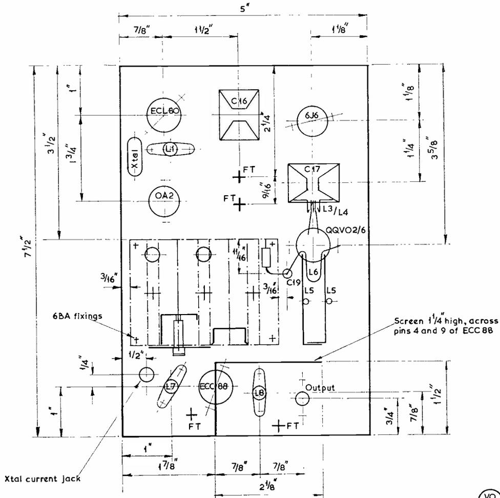
Fig. 2: DRILLING DIAGRAM 13cm CONVERTER
