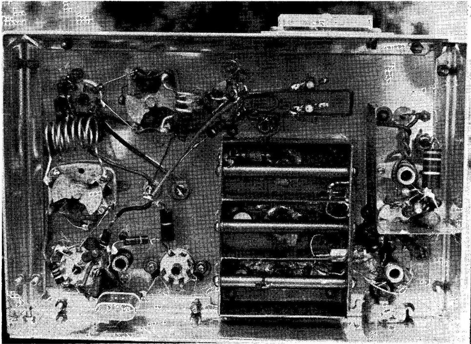
Under-chassis layout of the Converter—compare with drawing opposite of trough-line arrangement.
