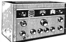
Latest release by ministry BRAND NEW in original cases. 110-250v. A.C. operation. Frequency in 6 Bands. 535 Kc/s.-32 Mc/s. continuous output impedance 2.5-600 ohms. Incorporating crystal filter, noise limiter, variable BFO, variable selectivity, etc. Price: £87/10/-, Carr. £2.
