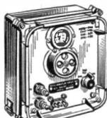
Small portable crystal controlled wavemeter. Size 7 x 7 1/2 x 4 1/2 in. Frequency range 500 Kc/s.-10 Mc/s. (up to 30 Mc/s. on harmonics). Callibrated dial. Power requirements 300v. DC. 15mA and 12v. DC 0-3A. Excellent condition, 89/6. Carr 7/6.
