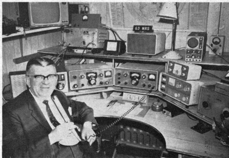
The very well-appointed and laid out station of G3NRS, Stanley Scales, 17 Westfield Avenue, Scarborough, Yorkshire, who runs the Collins S-Line-75S-3 Rx and 32S-3 Tx—with a KW-600 Linear and a Star SR-200 receiver (incorporating converter for Two). His antennae consist of a Tri-Band rotary Quad on a 40ft. tower and a K.W. trap dipole for general coverage.
