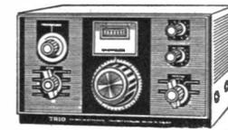
7 separate ranges between 3.5 and 29.7 Mc/s. 7 valves, 2 transistors and 5 diodes plus 8 crystals: output 8 and 500 ohm and 5000 ohm phone jack. Crystal controlled oscillator. Variable BFO. VFO. AVC. ANL. 5 meter. SSB-CW. Stand-by switch special double gear dial drive socket for connection to a transmitter. 115/250v. A.C. Mains. Size: 7" x 13" x 10" with instruction manual and service data, £65.00, Carriage paid. Package deal: JR500SE with SP5D speaker and H54 headphones, £69.50.
