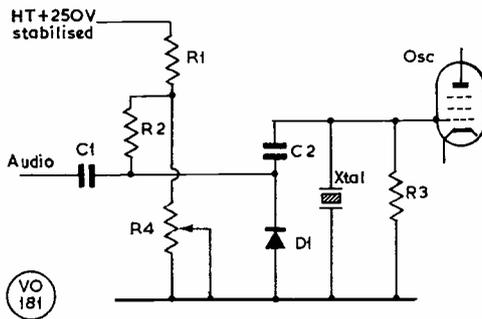
Circuit of the NBFM arrangement for application to the CO of an existing crystal-controlled transmitter. Values can be: C1, .01  $\mu$ F; C2, 10-20  $\mu$ F; R1, 270K; R2, 100K; R3, 47K; R4, 47K potentiometer set at suitable bias voltage for diode used. D1 can be REC-53, BY-100 or similar. For notes on deviation, see "VHF-UHF Manual".
