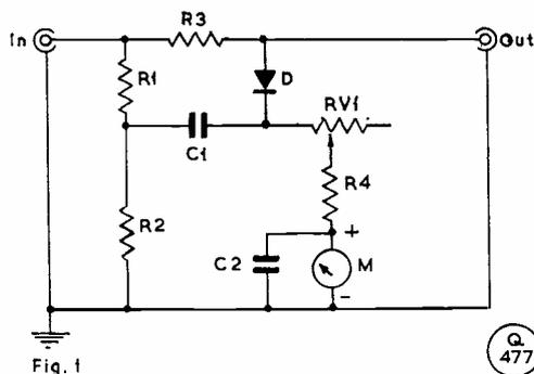
Fig. 1. Circuit of the SWR bridge, for which values can be: R1, R2, 47 ohms, rated 5 watts; R3, 68 ohms, 10-watt; R4, 1000 ohms,  $\frac{1}{2}$ -watt. C1, C2, .005  $\mu$ F; D, any small diode; meter, 0-500  $\mu$ A. Note that R1, R2, could each be made up of five 240-ohm 1-watt resistors in parallel, and R3 ten of 680 ohms, rated 1 watt. Potentiometer RV1, for setting, is 25,000 ohms.
