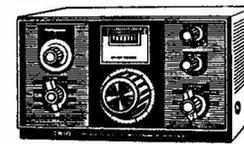
7 separate ranges between 3.5 and 29.7 Mc/s. 7 valves, 2 transistors and 5 diodes plus 8 crystals: output 8 and 500 ohm and 5000 ohm phone jack. Crystal controlled oscillator. Variable BFO. VFO. AVC. ANL. 5 meter. SSB-CW. Stand-by switch. special double gear dial drive socket for connection to a transmitter. 115/250v. A.C. Mains. Size: 7" x 13" x 10" with instruction manual and service data, £65-00, Carriage paid. Package deal: JR500SE with SP5D speaker and HS4 headphones, £69-50.
