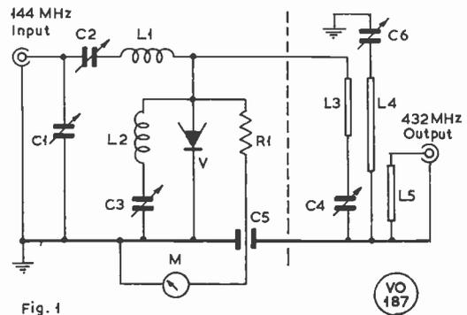
Fig. 1 Circuit of the 144-432 MHz varactor tripler, discussed in the text.
