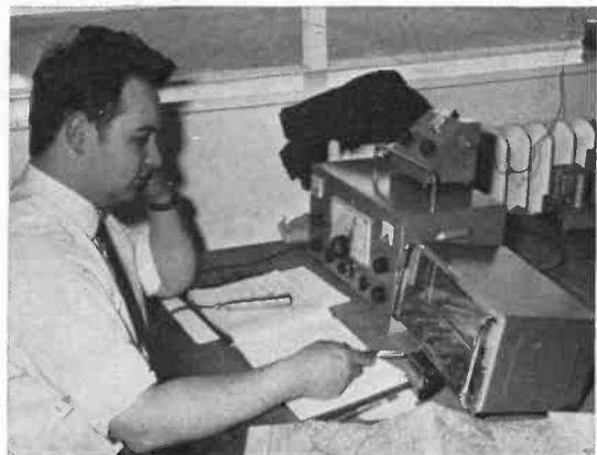
For the Northern Mobile Rally, the Top Band talk-in station signed G3WVD/A, with a home-built transceiver operated by G3MFJ. He had an EC-10 as stand-by Rx.
