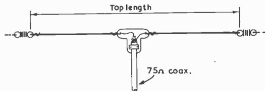
Fig. 1 Important dimension of a dipole
