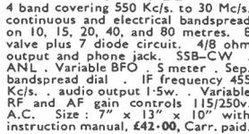
4 band covering 550 Kc/s. to 30 Mc/s. continuous and electrical bandspread on 10, 15, 20, 40, and 80 metres. 8 valve plus 7 diode circuit. 4/8 ohm output and phone jack. SSB-CW. ANL. Variable BFO. 5 meter. Sep. bandspread dial. IF frequency 455 Kc/s. audio output 1.5w. Variable RF and AF gain controls 115/250v. A.C. Size: 7" x 13" x 10" with instruction manual, £42-00. Carr. paid.
