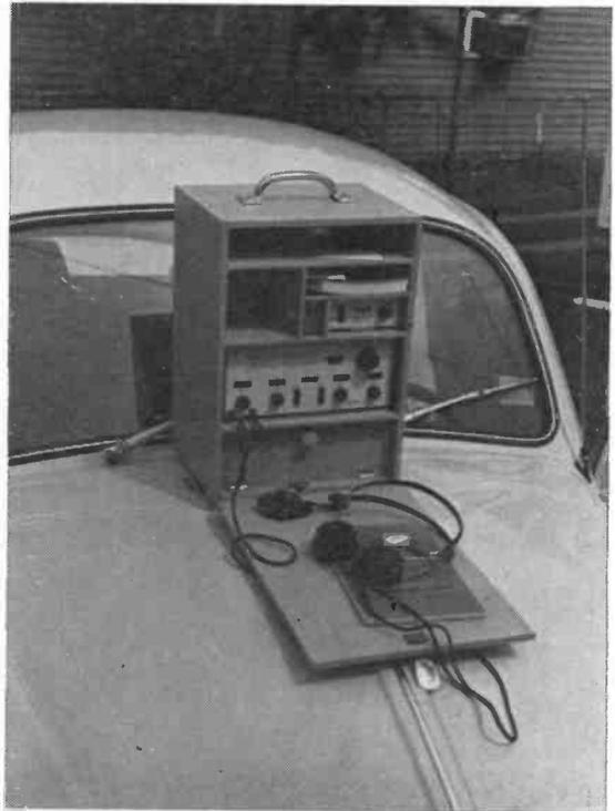
If ever you hear or work W5TVW-suffixed, this is the little rig he carries about with him—a Ten-Tec 20/40m. QRP outfit in a home-made plywood cabinet, with accommodation for the ancillaries, including cut-wires for dipole antennae, logs, etc. Operation with this 5-watt solid-state Tx/Rx is on CW, the aerial being strung up to any convenient support. That's the way to work /P with a mobile rig. The QSL address for W5TVW is Elliot Blaize, 600 Deckbar Avenue, New Orleans, 70121, Louisiana, U.S.A.
