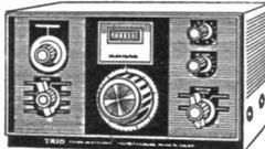
7 separate ranges between 3-5 and 29-7 Mc/s. 7 valves, 2 transistors and 5 diodes plus 8 crystals: output 8 and 500 ohm and 5000 ohm phone jack. Crystal controlled oscillator. Variable BFO. VFO. AVC. ANL. 5 meter. SSB-CW. Stand-by switch. special double gear dial drive socket for connection to a transmitter. 115/250v. A.C. Mains. Size: 7" x 13" x 10" with instruction manual and service data, £65-00. Carriage paid. Package deal: JR500SE with SP5D speaker and H54 headphones, £69-50.
