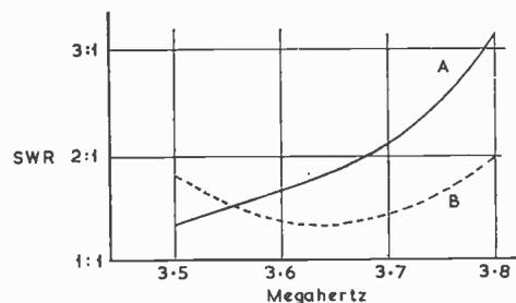
Fig. 2 Effect of length on SWR
