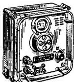
Small portable crystal controlled wavemeter. Size 7" x 7 1/2" x 4". Frequency range 500 Kc/s.-10 Mc/s. (up to 30 Mc/s. on harmonics). Calibrated dial. Power requirements 300v. D.C. 15mA and 12v. D.C. 0.3A. Excellent condition, £4.47 1/2. Carr. 37p.
