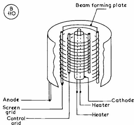
Fig. 5 Construction of a Beam Tetrode (see text).
