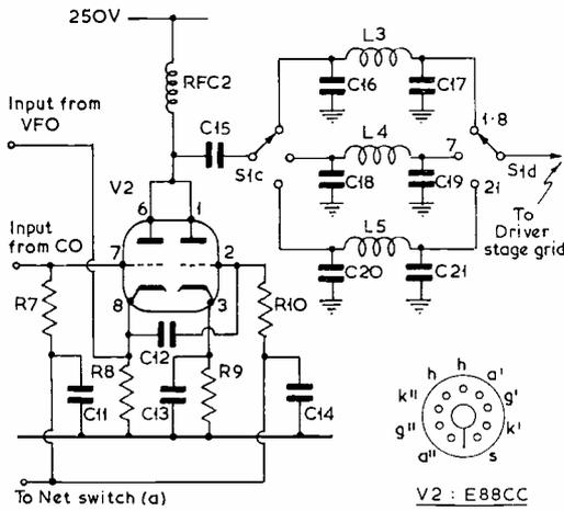
Fig. 3 Diagram of Mixer stage
