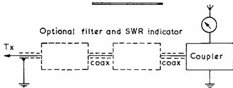
Fig. 2 Position of Meter with End-fed aerial
