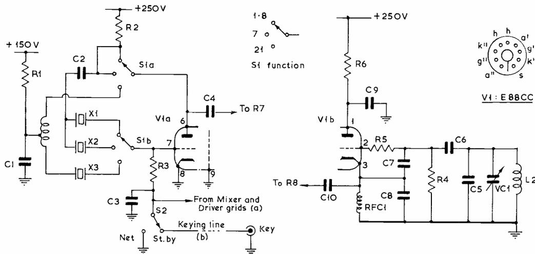
Fig:2 Crystal Oscillator and VFO stages
