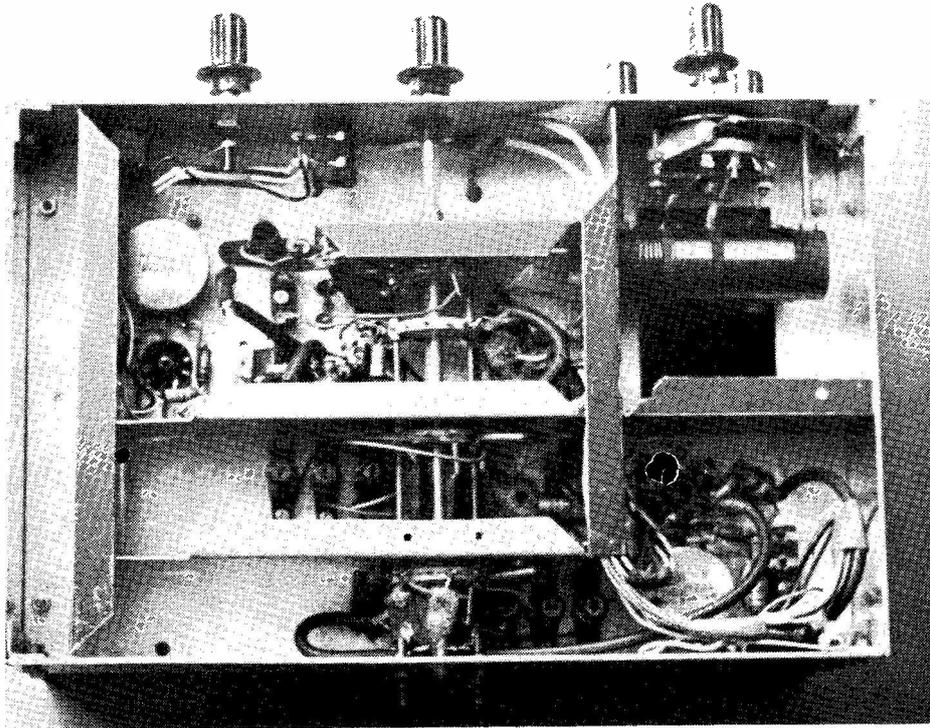
The general construction under-chassis for the transmitter as built by GM3NHQ. The generous screening is an important factor in attaining stability and generally consistent operation. The screens are flanged so that the bottom plate can be bolted to them using self-tapping screws.
