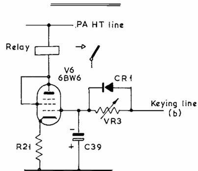
Fig. 6b Revised Receiver Muting circuit
