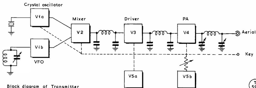
Fig. 1 Block diagram of Transmitter
