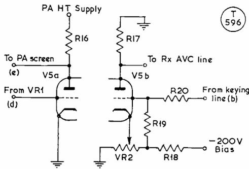
Fig. 5 The Muting and Power Control stages
