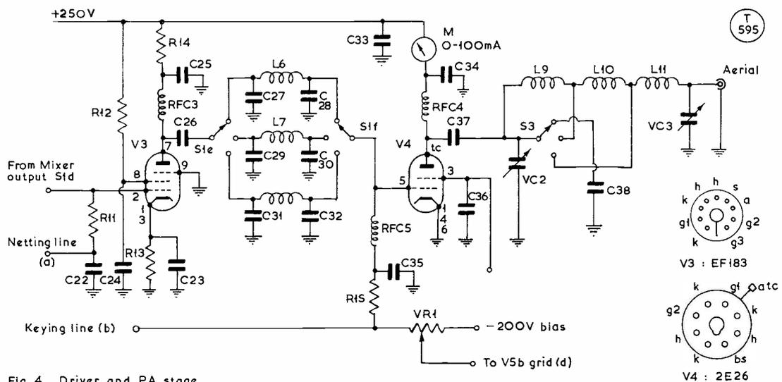
Fig. 4 Driver and PA stage
