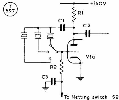
Fig. 6a Modified Oscillator circuit
