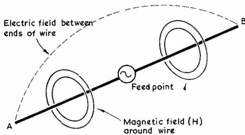
Fig. 2 a. Simple centre-fed dipole showing Electric and Magnetic fields
