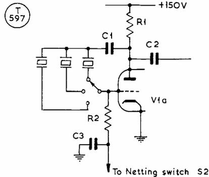
Fig. 6a Modified Oscillator circuit
