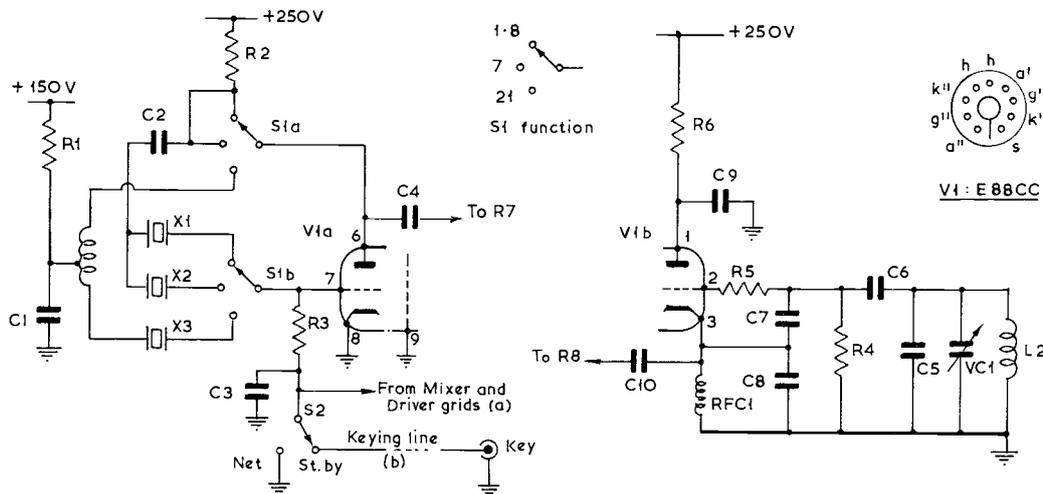
Fig:2 Crystal Oscillator and VFO stages
