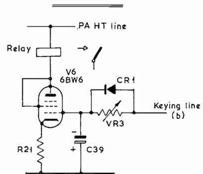
Fig. 6b Revised Receiver Muting circuit
