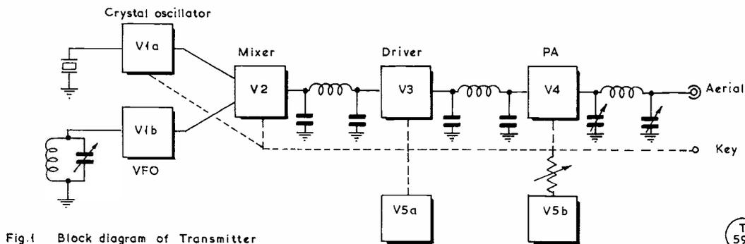
Fig. 1 Block diagram of Transmitter
