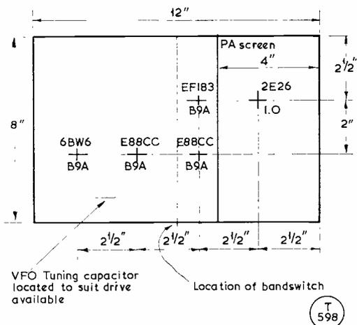
Fig. 7. Chassis plan upper-side, with location of main items.
