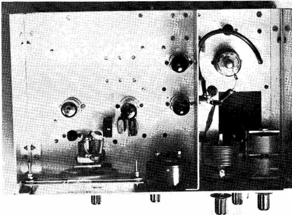
Upper-side view of the chassis layout. The VFO tuning capacitor should be positioned to suit whatever dial mechanism is chosen—in this case it was home-constructed. The large cut-out in the PA compartment should be ignored!
