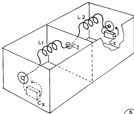
Fig. 1c Construction of Rudimentary Filter
