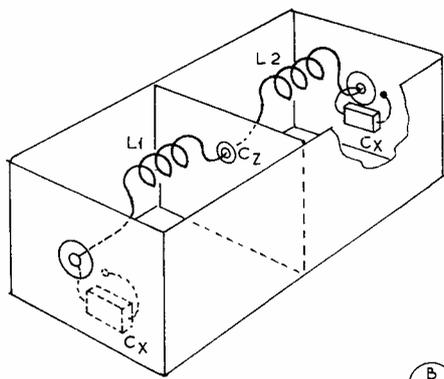
Fig. 1c Construction of Rudimentary Filter
