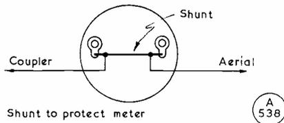
Fig. 3 Shunt to protect meter
