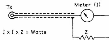
Fig. 1 Calculating RF Power with the Meter
