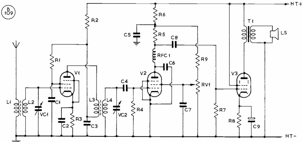
Fig. 4 Circuit Diagram of Three Valve TRF Receiver
