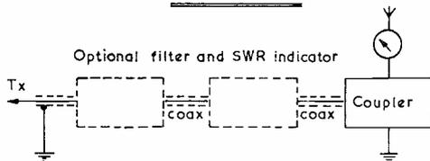
Fig. 2 Position of Meter with End-fed aerial
