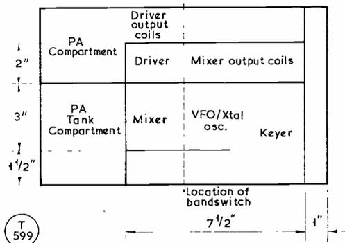
Fig. 8. Inter-stage screening, underside of chassis.
