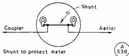
Fig. 3 Shunt to protect meter
