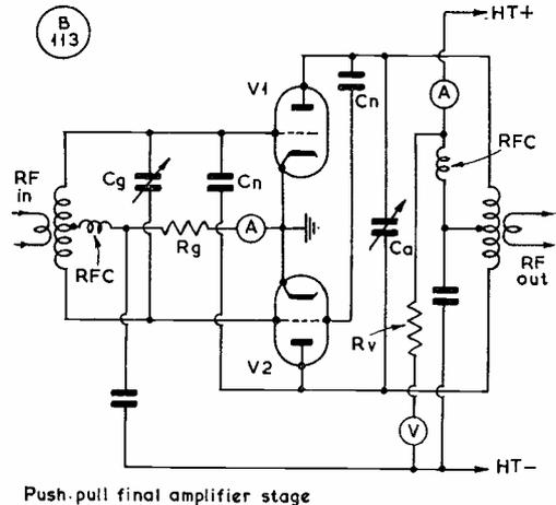
Fig. 8. (To answer Q.10). A push-pull RF stage, cross-capacity neutralised, Cn, and having grid current, anode current and anode volts measured. The use of these is discussed in the text.
