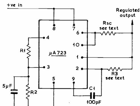
Fig. 3 a. Basic Low Voltage Regulator +2 to 6volts
