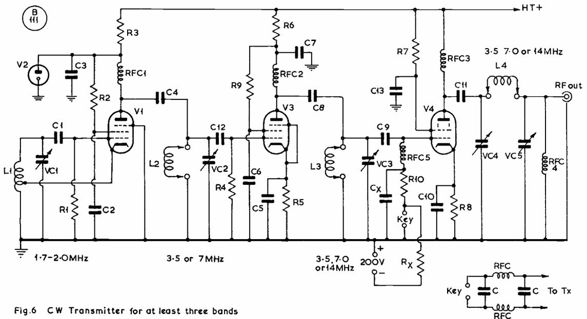
Fig.6 CW Transmitter for at least three bands
