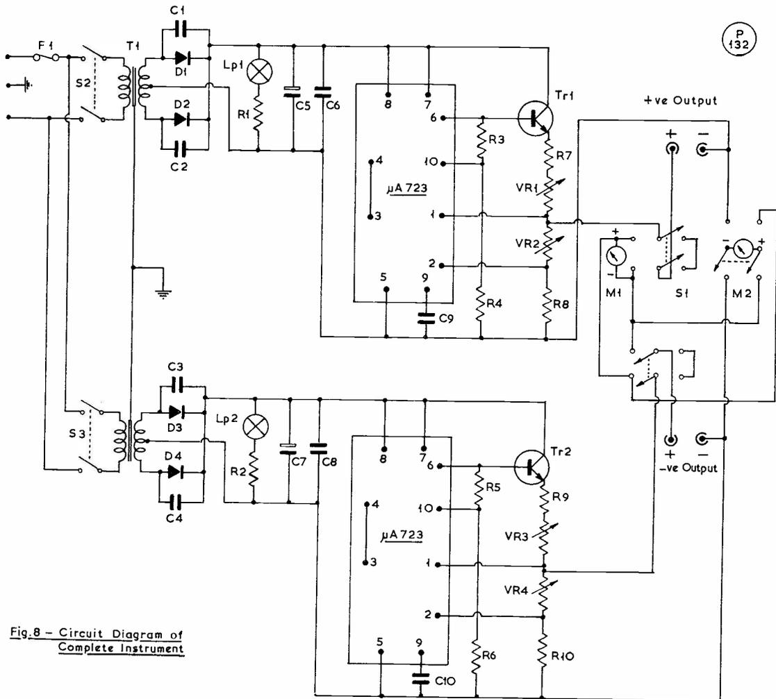
Fig.8 - Circuit Diagram of Complete Instrument
