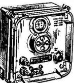
Small portable crystal controlled wavemeter. Size 7" x 7" x 4". Frequency range 500 Kc/s.-10 Mc/s. (up to 30 Mc/s. on harmonics). Calibrated dial. Power requirements 300v. D.C., 15mA and 12v. D.C. 0-3A. Excellent condition, £4-47½. Carr. 37½p.
