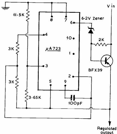
Fig. 6 - Typical Negative Voltage Regulator
