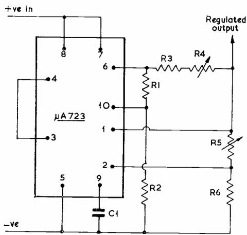
Fig. 5 - High Voltage Regulator with Foldback Current Limiting
