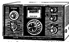
7 separate ranges between 3-5 and 29-7 Mc/s. 7 valves. 2 transistors and 5 diodes plus 8 crystals: output 8 and 500 ohm and 5000 ohm phone jack. Crystal controlled oscillator. Variable BFO + VFO + AVC + ANL + S meter + SSB-CW + Stand-by switch + special double gear dial drive socket for connection to a transmitter. 115/250v. A.C. Mains. Size: 7" x 13" x 10" with instruction manual and service data, £65-00. Carriage paid. Package deal: JR500SE with SP5D speaker and HS4 headphones, £69-50.
