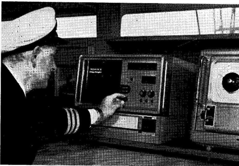
The new Redifon “Omega Navigator” receiver will give a ship positions accurate to within about one mile on ocean passages across the world. It is, of course, a satellite-referred device and is now installed in the new ship m.v. “Orbita” of the Pacific Steam Navigation Co., Ltd.
