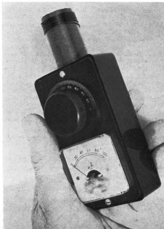
An indicating absorption wavemeter, using a plastic box as container to minimise hand-capacity effects, and an 0-100 microamp. m/c meter as the resonance indicator.
