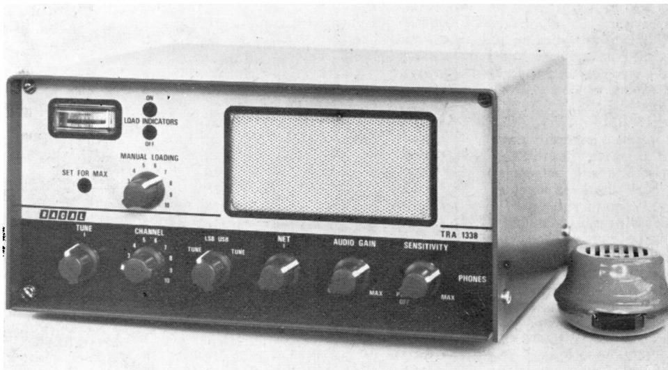
The new Racal-Mobilcal TRA.1338 is a commercial 25-watt SSB transceiver to cover a frequency range of 2.0 to 8.0 MHz, there being ten crystal channels which can be pre-set in that range. The design is solid-state, with output matching possible into virtually any type of aerial. Modes of operation are AM/CW/SSB and, being intended for mobile working, it is light and compact and runs off a 12v. negative-earth supply.
