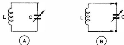
Fig.1 Absorption Wavemeters for one or several ranges
