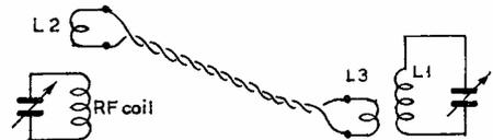
Fig.5 Coupling a Wavemeter with a link line
