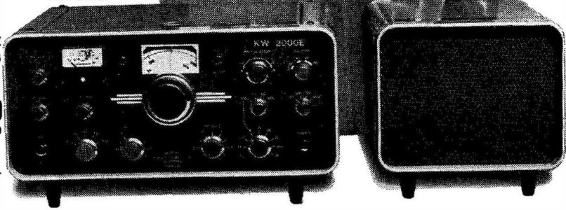
A KW 2000E with 500 kHz VFO COVERAGE 10-160 metres
