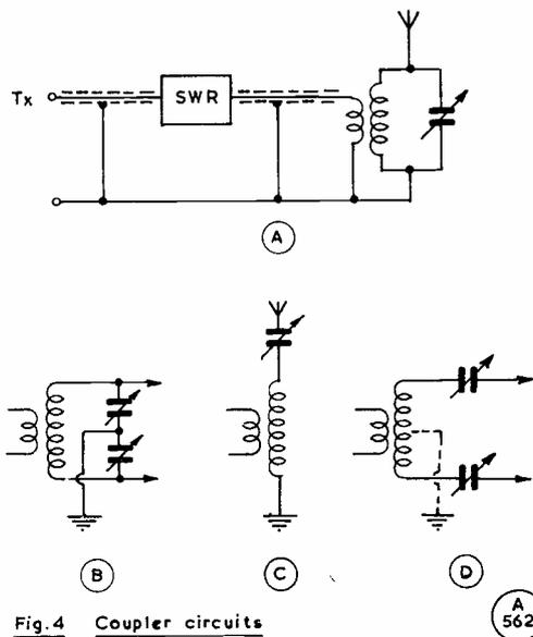
Fig. 4 Coupler circuits
