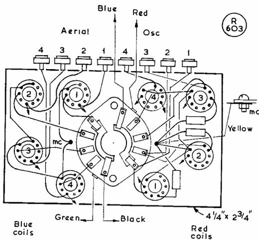
**Fig. 3. Wiring of the Coil pack**
