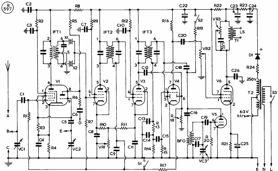
Fig. 2 Complete circuit of the Receiver
