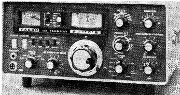
This is a new and improved version of the well-known FT101. It is fitted with a cooling fan as standard and is improved in several respects :—
