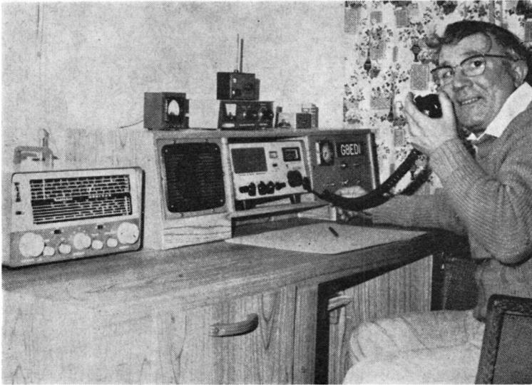
E. Waddington, G8EDI, 18 Barnwood Road, Earby, Colne, Lancs. has an HW-17 with FET pre-amp., all built into a neat console, with outside an 8-ele flat-top at 35ft. The Rx on the left is a Mohican GC-1U, the Heathkit full-coverage transistor receiver.
