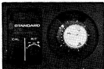
The CV110 is a remote VFO for the C140 Transceiver and has a centre tuning meter plus RIT ( $\pm 5$  kHz) and CAL tuning to accurately calibrate the VFO.
