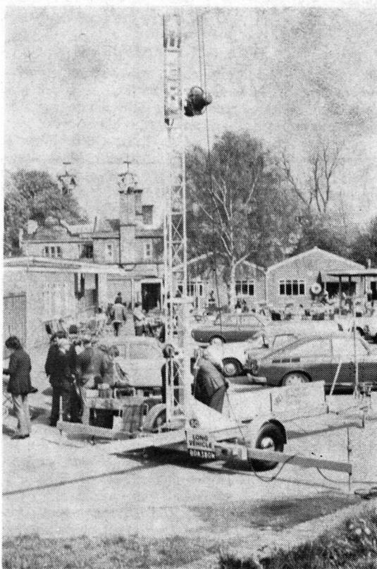
The Versatower installation used for the communication and talk-in stations at the North Midlands Rally. It is mounted on its own towing vehicle.
