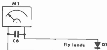
Values for the Test Oscillator/RF Sniffer can be: C1, C2, .001  $\mu$ F; C3, 10  $\mu$ F trimmer; C4, 10  $\mu$ F silver mica; C5, 47  $\mu$ F 8/m; C6, 220  $\mu$ F, disc; R1, R6, 15K; R2, R5, 2.2K; R3, R4, 100 ohms; Tr1, Tr2, BC107; Coil, 5 turns 20g, to  $\frac{1}{4}$ -in. dia. And for the Sniffer, D1 is IN4148 or similar; M1, 0-500  $\mu$ A meter; and X1, 14 MHz crystal (see text).
