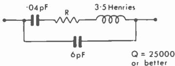
(b) Equivalent electrical circuit of 400kHz crystal.
