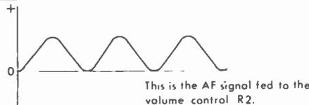
(c) The mean AF signal, after decoupling the RF component: junction R1, C2.
