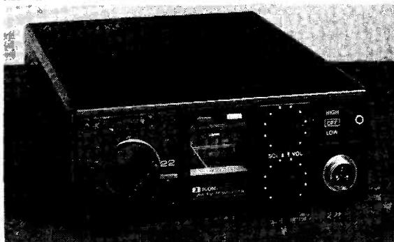
The IC-22A is becoming very popular as THE mobile rig for both simplex and repeater operation. See last month's advert for brief specification or contact us or one of our agents for more details. Fitted with an Automatic tone burst which operates on repeater channels only, the IC-22A comes fitted with 5 or 8 channels. The maximum number of channels available is of course 22.
