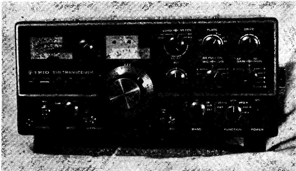
Front view of the Trio TS-520 Transceiver. A carrying handle is provided at the right-hand side of the cabinet, with some extra feet on the left panel drop, so that it can be carried and set down just like a brief-case.
