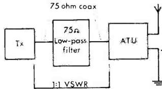
(b) Installation of Low-pass filter
