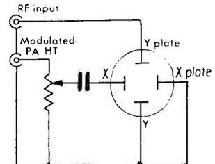
(f) Over-modulation indicator using oscilloscope
