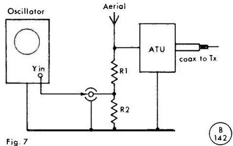
Fig. 7, to go with Q.9. It should be noted that, if X and Y plates can be directly connected, the 'scope can be used, without time-base or amplifiers, as shown at Fig. 1F, to obtain a trapezoid pattern.
