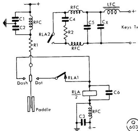
Fig. 2. The keyer circuit complete. Capacitors C1-C5 are all .001  $\mu$ F; C6 is 2  $\mu$ F; the value of Cx depends upon several factors—see text. R1 is 10,000 ohms for a 240v. DC supply and a relay of 10,000 ohms; R2 is 1000 ohms. All RF chokes are standard 2.5 mH. C6 can be varied (by switching) from 0.5-2  $\mu$ F to change the dot speed. LFC is a 30-Hz. choke and the relay should be a G.P.O. type having one set of contacts closed (A1) and one pair open (A2) in the “rest” position.
