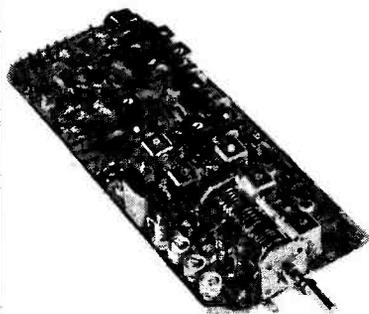
**AR10** Mosfet receiver. 28-30 MHz Double conversion superhet. RF and amplifier stages are gate protected mosfets for good sensitivity and low intermodulation. Noise limiter and squelch circuit. AM, SSB and CW reception. 12v. DC.
