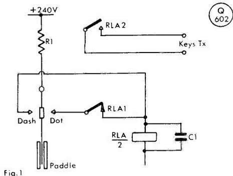
Fig. 1. Basic circuit for the auto-keyer. Dots are made automatically, depending upon the value of R1 and the capacity of C1. The relay can be a standard G.P.O. type of about 10,000 ohms resistance.
