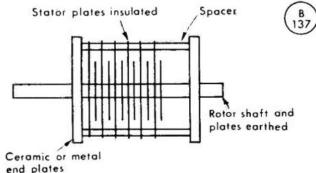
Fig. 2 Construction of a variable capacitor
