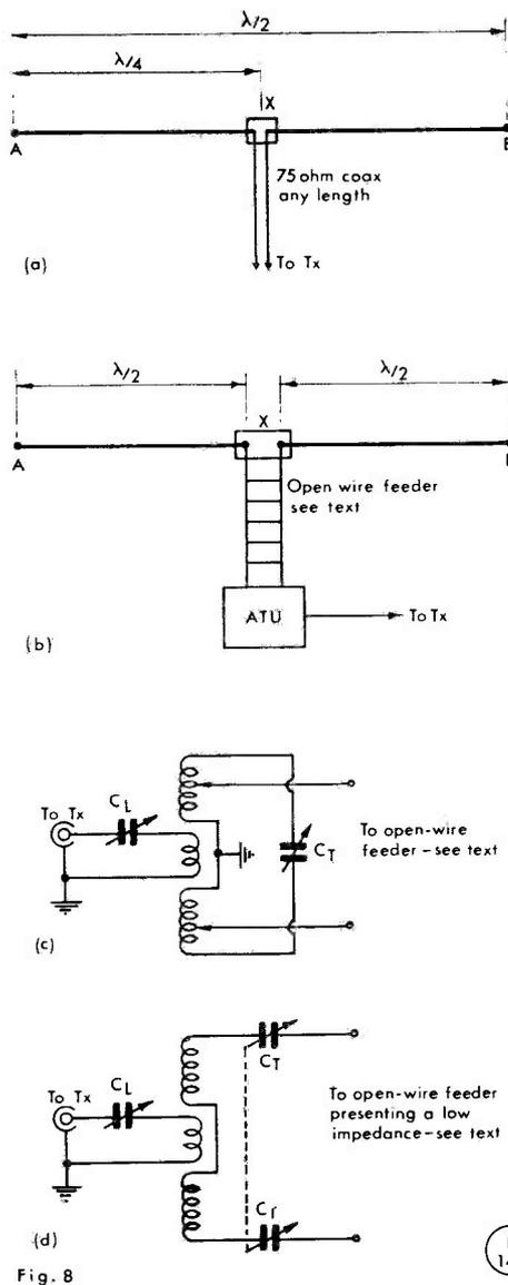
Fig. 8, to go with Q.10. (A) half-wave dipole, fed with coax. (B) full-wave dipole, centre-fed with open-wire matched line. (C) a normal ATU (aerial tuning unit) configuration. (D) ATU circuitry when a low impedance appears at the bottom of the feeder line.
