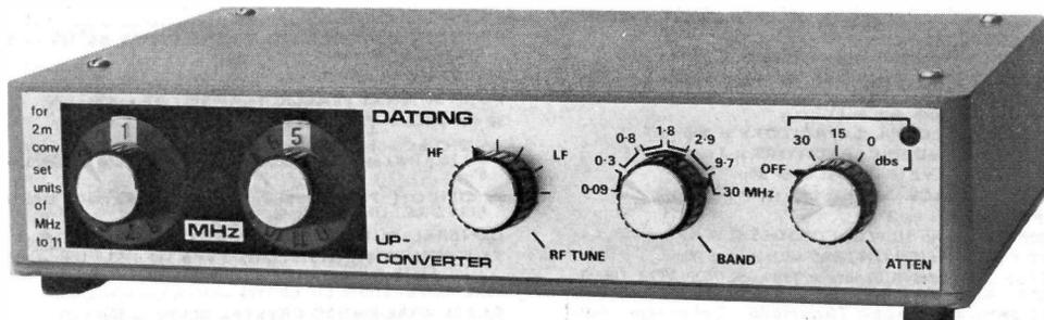
Model UC/1 converts any existing amateur-bands-only receiver which has coverage of 28-29 MHz or 144-145 MHz (e.g. HF bands receivers or transceivers and 2-metre "all-mode" transceivers) into a general coverage receiver with equivalent high performance. Compared with the alternative of purchasing a separate receiver for general coverage, Model UC/1 avoids wasteful duplication and gives better performance for less outlay.
