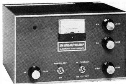
This Linear Amplifier has been developed by us to fill the need for a high power add-on unit for use mainly with low power SSB transverters. The unit also contains a low-noise receive preamplifier which is equipped with an RF gain control. Mains operated. Drive requirement : 5-20 watts. CW and SSB, 5 watts maximum AM & FM. P.A. 50% efficient. R.F. switched so no modification to transceiver is necessary.
