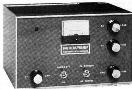
This Linear Amplifier has been developed by us to fill the need for a high power add-on unit for use mainly with low power SSB transceivers. The unit also contains a low-noise receive preamplifier which is equipped with an RF gain control. Mains operated. Drive requirement : 5-20 watts. CW and SSB, 5 watts maximum AM & FM. P.A. 50% efficient. R.F. switched so no modification to transceiver is necessary.
