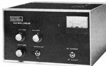
Following the success of our 432 MHz Linear Amplifier assembly EDL 432 and due to the increasing enquiries for a self contained unit, ELECTRONIC DEVELOPMENTS are pleased to announce the unveiling of a new linear filling these needs, the EDL 432P. This new unit utilizes the same P.A. as the EDL 432 and is complete with mains power supply, blower, aerial change over relays and full metering.
