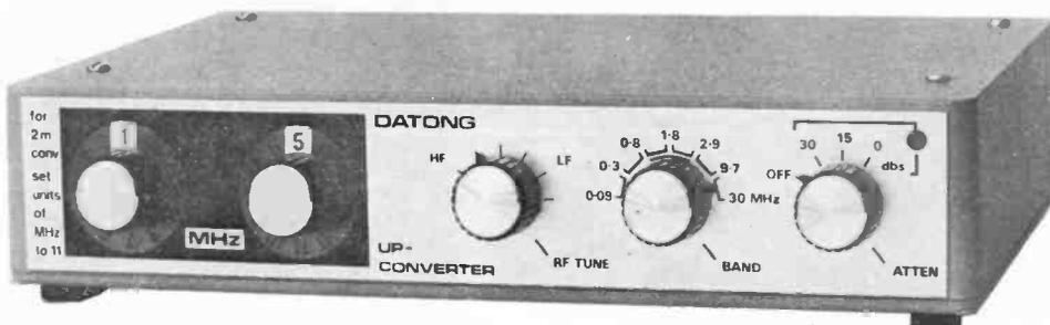
Model UC/1 converts any existing amateur-bands-only receiver which has coverage of 28-29 MHz or 144-145 MHz (e.g. HF bands receivers or transceivers and 2-metre "all-mode" transceivers) into a general coverage receiver with equivalent high performance. Compared with the alternative of purchasing a separate receiver for general coverage, Model UC/1 avoids wasteful duplication and gives better performance for less outlay.
