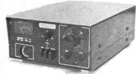
AK20. STE. Latest model from the famous STE Milan range of equipment. 12 channel operation in the 144-146 MHz range. 11-15v. DC operation. 8 watt output. Sensitivity 0.2 uv R.I.T. tone burst. Complete with microphone, and mobile bracket. Price £170 00
