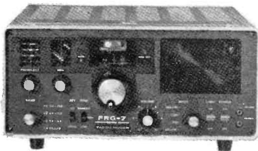
**YAESU FRG-7 RECEIVER.** Mains and battery operated receiver 0.5 to 30 MHz. Solid state. Advance circuitry offers excellent performance for the DX listener at a moderate price.
