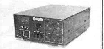
**AK20, 5TE.** Latest model from the famous STE Milan range of equipment: 12 channel operation in the 144-146 MHz range. 11-15v. DC operation. 3 watts output. Sensitivity 0.2 uv R.I.T. tone burst. Complete with microphone, and mobile bracket.
