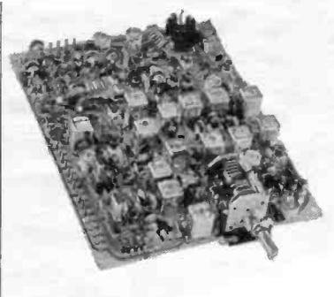
**AT222.** A complete transmitter exciter unit for 144-146 MHz on AM or FM. VFO controlled or fixed channel operation. Complete with microphone pre-amp., speech processor including active audio filter. 1 watt output. FM. .25 watt AM. Output impedance 50-75 ohm adjustable. Frequency deviation 3-10 kHz adjustable.
