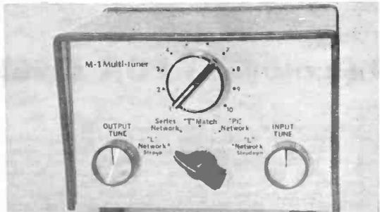
**Mk. 1 MULTI TUNER.** Designed and manufactured by us. 50 tunable switched positions for antenna lengths over 5 metres in the 2-30 MHz range. Five different circuits to give an excellent match between your receiver and antenna. Now in use in over 35 countries. Price £17.50. Including VAT and Postage.
