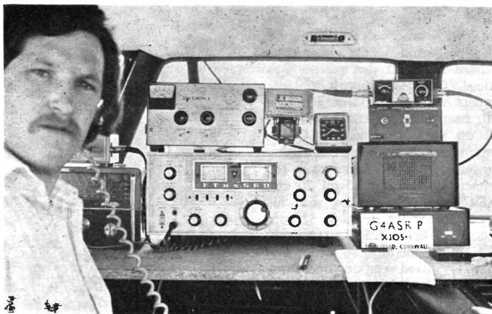
David Butler operating G4ASR/P during the May 2m. portable contest. The "prime-mover" was an FT-DX560 transceiver driving a Europa transverter feeding two bayed, 6-element, Jaybeam quads; additional punch to the signal was provided by a Datong RF speech processor. 432 stations were worked on 23cm., 70cm. and 2m. during the last three weeks in May from a rare "XJ" QTH square in Cornwall.
