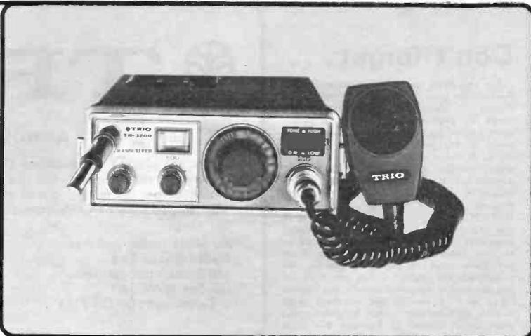
12 channel capability with three channels factory fitted with crystals for SUB, 18 and 20. Supplied with all accessories as the TR2200GX and including a new high gain 5/8 wave antenna.
