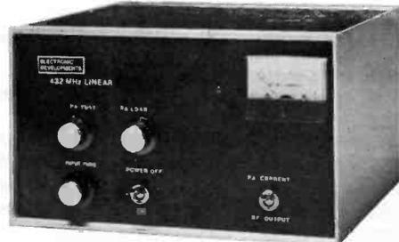
This new unit utilizes the same P.A. as the EDL 432 and is complete with mains power supply, blower, aerial change over relays and full metering. **PRICE : £151.90 (inc. VAT)**
