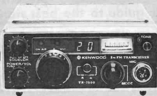
ensures a superbly clean signal with no unwanted multiplier products, and an all new PA system with specially developed transistors gives output powers well in excess of normal specifications.
