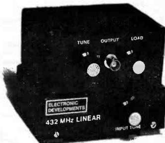
This 432 MHz Linear is operated in grounded grid configuration and exhibits a gain of typically 10dB. With a drive input of 5 watts its output power is in the order of 50 watts which is more than adequate for OSCAR 7. Power requirements are 6.3v. AC and H.T. 400-1000v. DC. Fitted with BNC connectors. **PRICE : £56.25 (inc. VAT)**
