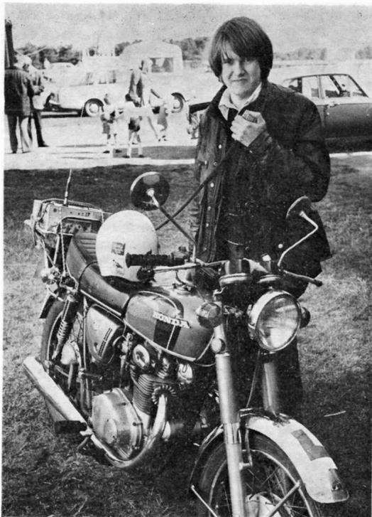
Mike Rhys, G8KTC, a member of the Torbay A.R.S. turned up at their Mobile Rally, at Haldon racecourse on August 28th, with this unusual 2m. mobile rig. With 5 watts FM, he can operate on the move as he has a mic. and phones built into his helmet and a send/receive switch on the handlebars.
