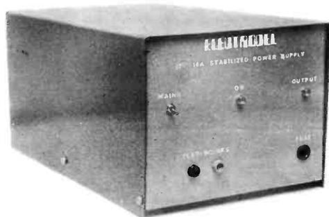
This unit will power your mobile rig or any other equipment including charging batteries. It is short circuit proof and protected against thermal overload. Substantial RF filtering is provided and the output voltage is adjustable over the range 11 to 14.5v.
