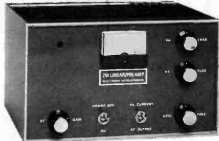
This Linear Amplifier has been developed by us to fill the need for a high power add-on unit for use mainly with low power SSB transceivers. The unit also contains a low-noise receiver preamplifier which is equipped with an RF gain control. Mains operated. Drive requirement : 5-20 watts. CW and SSB, 5 watts maximum AM & FM. P.A. 50% efficient. R.F. switched so no modification to transceiver is necessary. **PRICE : £151.90 (inc. VAT)**
