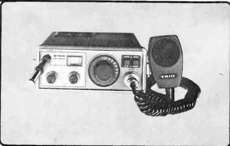
12 channel capability with three channels factory fitted with crystals for SUB, 18 and 20. Supplied with all accessories as the TR2200GX and including a new high gain 5/8 wave antenna. Don't forget, the following accessories are provided with the TR2200GX and TR3200 —
