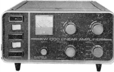
Decca KW 1000 Linear Amplifier for SSB and CW 10-80 metres, 1200 watts p.e.p. Input SSB, can be "driven" by most 100 watt Transceivers and Transmitters. Employs a pair of 1160L Tubes in grounded grid. Pi-section input and output circuits. Built-in 2.4Kv P.S.U.
