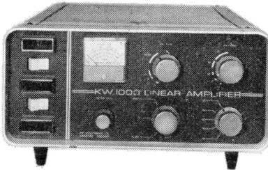
Decca KW 1000 Linear Amplifier for SSB and CW 10-80 metres, 1200 watts p.e.p. input SSB, can be "driven" by most 100 watt Transmitters and Transmitters. Employs a pair of T160L Tubes in grounded grid. Pi-section input and output circuits. Built-in 2.4Kv P.S.U.
