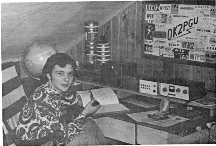
The mostly home-built 160m. station of Rostislav Pospisil, OK2PGU. Tx antenna is a 125-ft. vertical with a capacity hat, while a Beverage is used for receiving. Rosti, who already has 160/WAC, is aiming for DXCC/160—*with 48C/43 so far 'in the bag'.*
