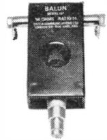
Decca-KW Balun Mk. II. The Decca-KW Balun is broadband—3 to 30 MHz, rated up to 2kW p.e.p. 1:1 Ratio 50 ohms "unbalanced" feed to "balanced" output. Waterproof moulded case. Suitable for dipoles and Beam aerials.
