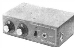
Processes speech as a SSB signal at 60 kHz to increase its ratio of average to peak levels without adding harmonic distortion. Improves talk power of SSB, FM, and AM transmitters without increasing the peak transmitted power. Connects between microphone and transmitter. (See articles by Dr. D. A. Tong, *Wireless World* Feb. 1975, 79-82 and Oct. 1976, 77-81.)
