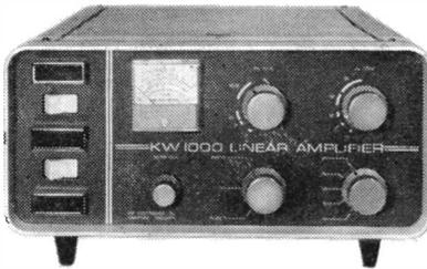
Decca-KW 1000 Linear Amplifier for SSB and CW 10-80 metres, 1200 watts p.e.p. input SSB, can be "driven" by most 100 watt Transmitters and Transmitters. Employs a pair of 1160L Tubes in grounded grid. Pi-section input and output circuits. Built-in 2-4Kv P.S.U.
