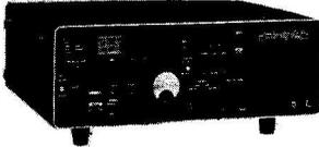
The FRG7000 is a digital readout, to 1 kHz, general coverage receiver which inclusively covers 250 kHz to 30 MHz. The receiver is sensitive (0.7 $\mu$ V for 10dBs(N) and very stable. Selectivity is switchable;  $\pm 1.5$  kHz for CW/SSB and  $\pm 3$  kHz (at -6dB) for AM. A digital clock is incorporated (settable to local and GMT time with a relay timer circuit (for switching on tape recorder etc).
