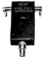
**Decca-KW Balun Mk. II.** The Decca-KW Balun is broadband—3 to 30 MHz, rated up to 2kW p.e.p. 1 : 1 Ratio 50 ohms "unbalanced" feed to "balanced" output. Waterproof moulded case. Suitable for dipole and Beam aeriels.
