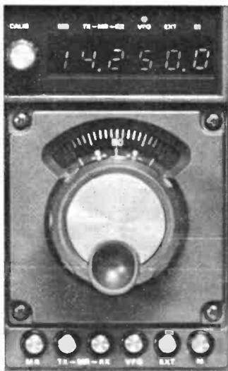
Offset tuning for either transmit or receive frequency allows precise zeroing in on that rare DX.
