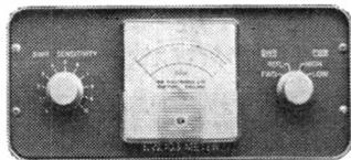
Decca KW-103 Combined Swr/Rf Power Meter is an instrument for measuring a 50 ohm coaxial line feeding an Aerial System or Dummy Load (1) Standing Wave Ratio, (2) RF Power with two ranges 0-100 & 0-1000W when used with a 50 ohm Dummy Load.
