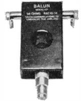
**Decca-KW Balun Mk. II.** The Decca-KW Balun is broadband—3 to 30 MHz, rated up to 2kW p.a.p. 1:1 Ratio 50 ohms "unbalanced" feed to "balanced" output. Waterproof moulded case. Suitable for dipole and Beam aeriars.
