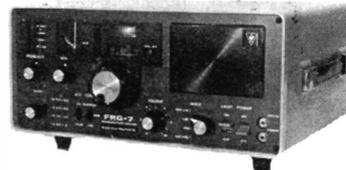
**YAesu FRG-7 RECEIVER.** Mains and battery operated receiver 0.5 to 30 MHz. Solid state. Advance circuitry offers excellent performance for the DX listener at a moderate price. Price £210-50
